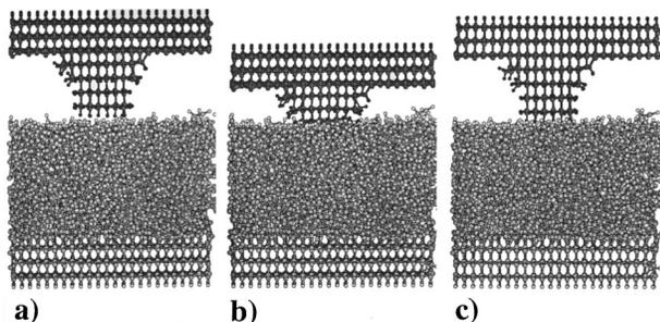
FIG. 3. Snapshots from a simulation where an amorphous-carbon film is indented by a  $sp^3$  bonded tip. The dark gray spheres are the carbon atoms in the tip, the light gray spheres are the carbon atoms in the film, the white spheres represent surface hydrogen atoms, and the black spheres represent tip hydrogen atoms. (a) Time=0.0 ps, (b) time=8.0 ps, (c) time=14.9 ps.
