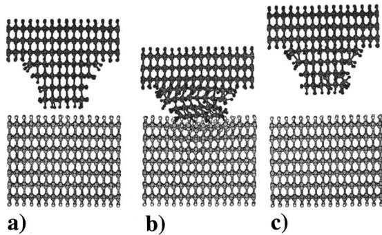
FIG. 1. Snapshots from a simulation where a diamond (111) surface is indented by a  $sp^3$  bonded tip. The dark gray spheres are the carbon atoms in the tip, the light gray spheres are the carbon atoms in the surface, the white spheres represent surface hydrogen atoms, and the black spheres represent tip hydrogen atoms. (a) Time=0.0 ps, (b) time=6.0 ps, (c) time=15.0 ps.
