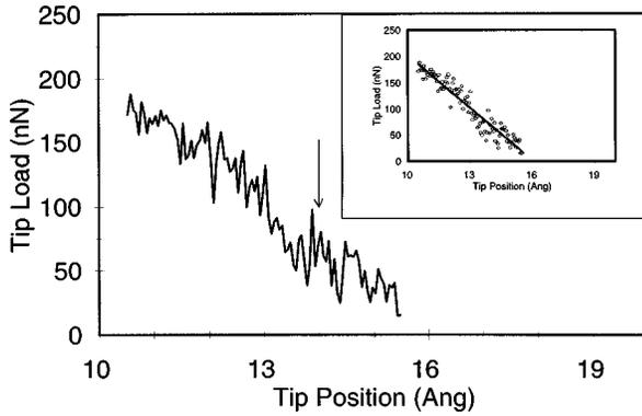
FIG. 2. Force on the tip vs distance of the tip for the indentation of the diamond (111) surface. Only the loading portion of the curve is shown. The arrow indicates the point where the tip first touches the surface. The inset shows the line of best fit to the data.
