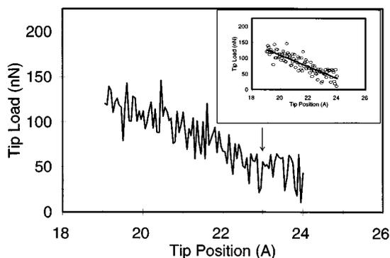
FIG. 4. Force on the tip vs distance of the tip for the indentation of the amorphous-carbon thin film. Only the loading portion of the curve is shown. The arrow indicates the point where the tip first touches the film. The inset shows the line of best fit to the data.
