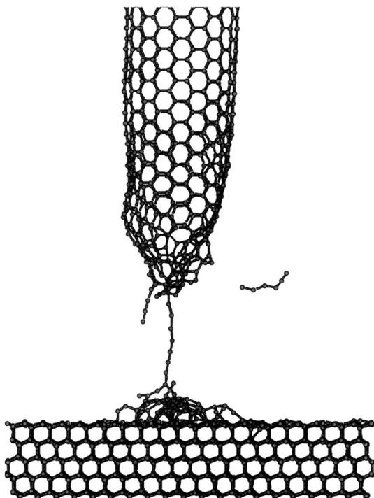
FIG. 3. Snapshot from a simulation where a capped 8.1-nm-long CNT tip indented and adhered to a C(111):C surface.
