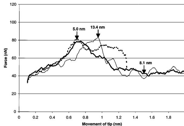
FIG. 2. Force-distance curves for capped CNT tips indenting C(111):H surfaces.
