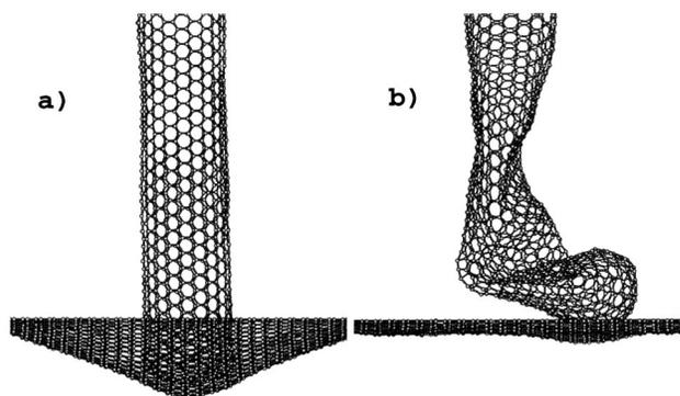
FIG. 4. Snapshots from simulations where capped CNT tips indented graphene sheets. (a) Deformation of the sheet as a capped 8.1-nm-long CNT tip presses against it, and (b) the tip has buckled and slipped.
