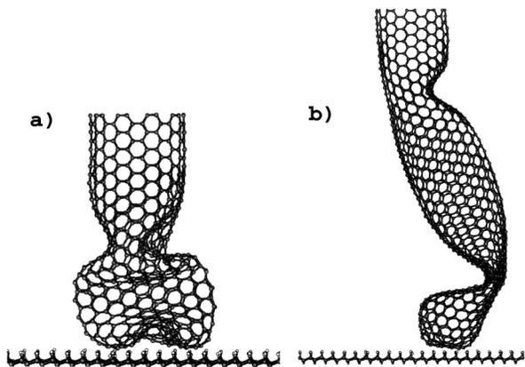
FIG. 1. Snapshots from simulations where capped CNT tips indented C(111):H surfaces. (a) Buckling and cap inversion for a 5.0-nm-long CNT tip, and (b) two buckles with some slip for a 8.1-nm-long CNT tip.
