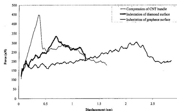
FIG. 5. Force curves for the nanotube rope during compression in free space, against a hydrogen-terminated, diamond (111) surface and against a graphite sheet.
