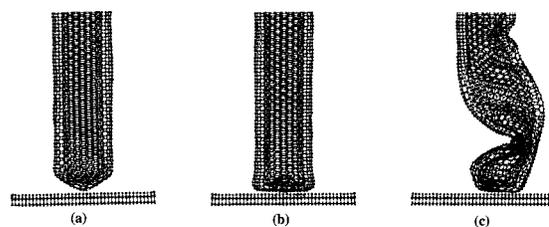
FIG. 1. Snapshots of the indentation of an 8.1 nm-long, capped multiwalled tubule on the C(111):H surface. The tubule consists of a (10,10) tube inside a (15,15) tube. (a) Starting configuration, (b) inversion of the inner and outer caps, and (c) slip after buckling twice.
