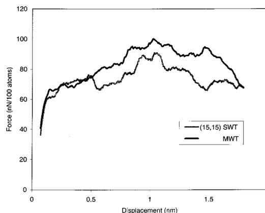
FIG. 2. Force curve from the indentation of a capped multiwalled tubule that consists of a (10,10) tube inside a (15,15) tube, and a single-walled (15,15) tube on the C(111):H surface.
