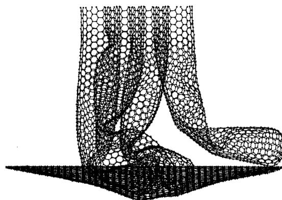
FIG. 4. Snapshot from the indentation of a rope of four capped (10,10) tubules against a graphene sheet during the pull-back phase. The tubule on the far right buckled twice on indentation while the others buckled only once. The figure shows how the rope end is distorted as a result of the indentation.
