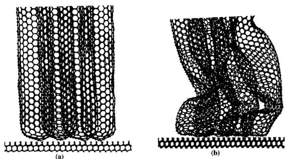
FIG. 3. Snapshots from the indentation of a rope of four capped (10,10) tubules against the C(111):H surface. (a) is the starting configuration and (b) is after buckling.
