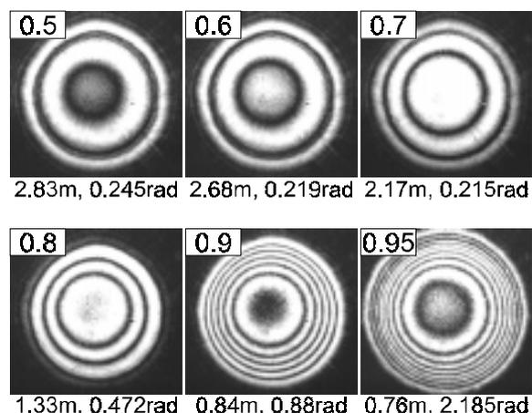
Fig. 9. Interferograms obtained using different duty cycles for bipolar rectangular control voltages with 9 V amplitude and 4 kHz frequency:  $q$  is indicated in the top-left corner of each interferogram. The resultant focal length and the rms phase deviation from an ideal parabola are shown on each lower insert.
