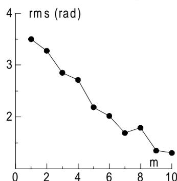
Fig. 3. Dependence of the rms phase deviation from an ideal parabola versus number of harmonic components  $m$  in the control signal  $U_0 \sum_{k=1}^m \alpha_k \sin(\omega_k t)$  for  $F = 0.6$  m.
