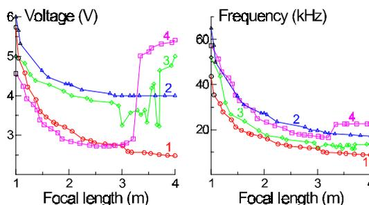
Fig. 6. Optimal control voltage parameters for different experimental samples of MLCL. 1,2,3,4 are for four different lenses.
