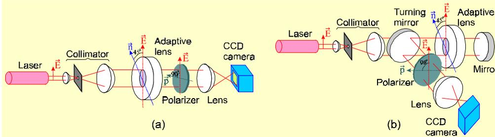
Fig. 4. Optical set-up for calibration of MLCL using (a) single pass and (b) double pass of collimated laser beam through LC layer:  $\vec{E}$  is direction of laser beam polarization,  $\vec{n}$  is initial alignment of LC molecules,  $\vec{p}$  is direction of polarizer orientation.
