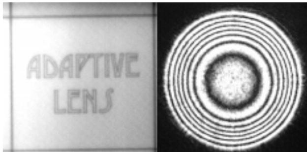
Fig. 10. (507 KB) Correction of defocus by a MLCL (left) and the corresponding interferogram variation (right).
