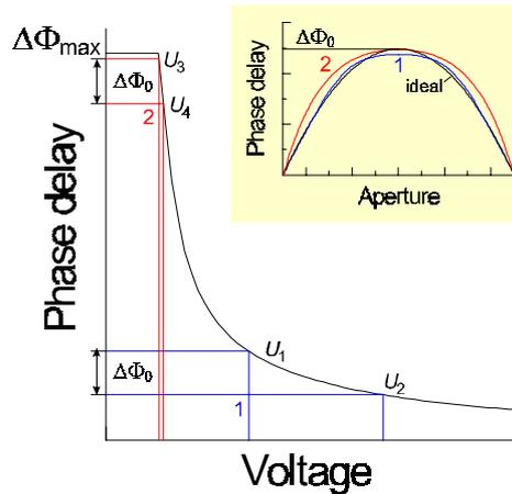
Fig. 7. Demonstration of lack of uniqueness in the definition of the optimal control voltage parameters.
