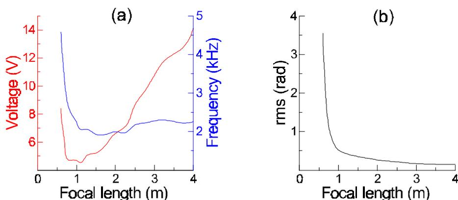
Fig. 2. (a) Theoretical dependence of the optimal control voltages and frequencies versus focal length for a modal liquid crystal lens. (b) Dependence of the rms phase deviation from an ideal parabola versus focal length.
