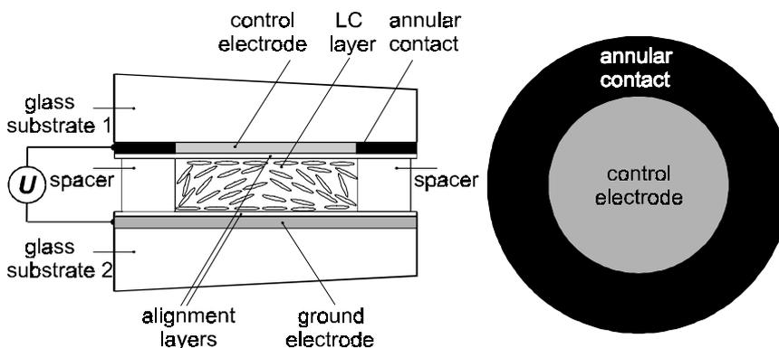
Fig. 1. A spherical modal liquid crystal lens.
