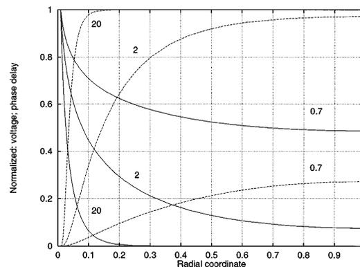
Fig. 3. Calculated normalized voltage distributions (solid curves) and phase delays (dashed curves) for three values of  $|\chi|$ .
