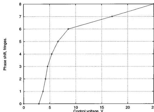
Fig. 2. Experimentally measured electro-optical characteristics of the LC cell.
