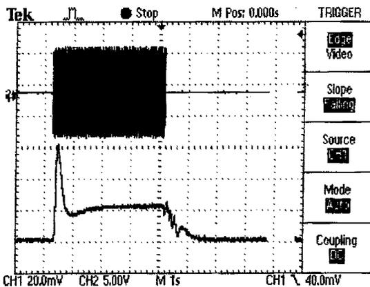
Fig. 8. Optically measured large-signal response (bottom curve) of the LC modulator to a 17.5-V (peak to peak) 75-kHz control voltage applied to a single actuator (top curve).
