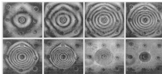
Fig. 5. Influence functions at constant control voltage  $U_0 = 7.5$  V and several control frequencies: 10, 20, 50, and 100 kHz (top, left to right) and 150 kHz, 250 kHz, 500 kHz, and 1 MHz (bottom, left to right). At low frequencies the influence function is so wide that only the central fringes are visible in the interferogram.
