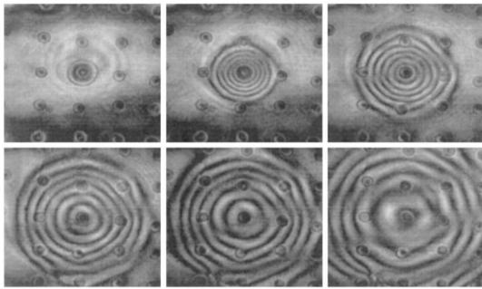
Fig. 6. Influence functions at a control frequency at 75 kHz at several control voltages: 5, 7.5, and 10 V (top, left to right) and 12.5, 15, and 20 V (bottom, left to right).
