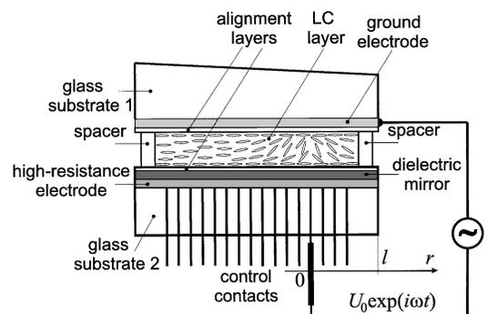
Fig. 1. Schematic diagram of a multichannel reflective LC phase corrector.
