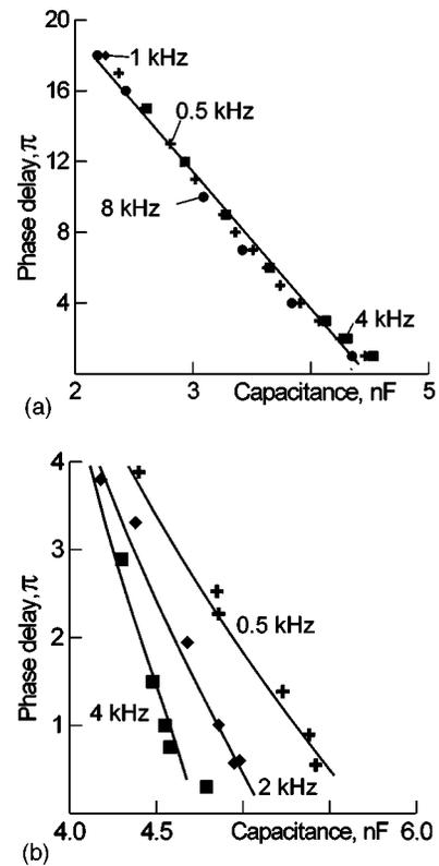
FIG. 4. Phase delay  $\Delta\Phi$  vs cell capacitance at different frequencies for (a) LC1348 and (b) LC1001.
