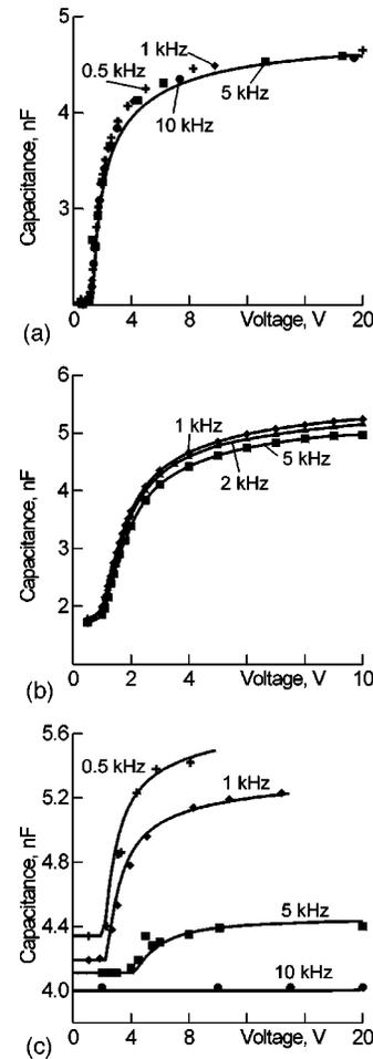
FIG. 2. Alternating Current voltage dependence of the cell capacitance at different frequencies for (a) LC1348, (b) E49 and (c) LC1001. The numbers in the plots denote frequency values.
