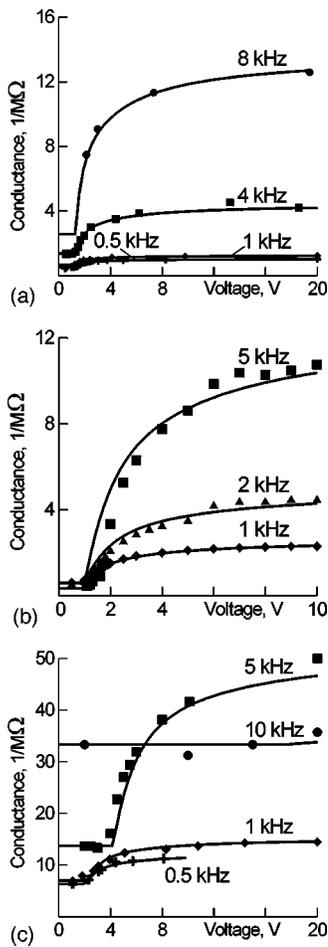
FIG. 3. Alternating Current voltage dependence of the cell conductance at different frequencies for (a) LC1348, (b) E49 and (c) LC1001.
