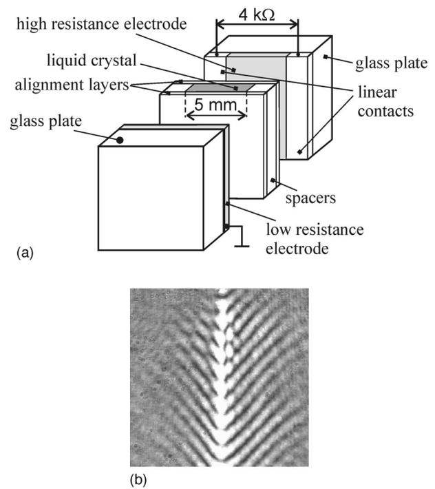
FIG. 7. (a) Schematic design of a MLCC with linear equidistant electrodes and (b) interferogram for frequency corresponding to dielectric constant dispersion:  $f = 870$  kHz,  $V = 4$  V.
