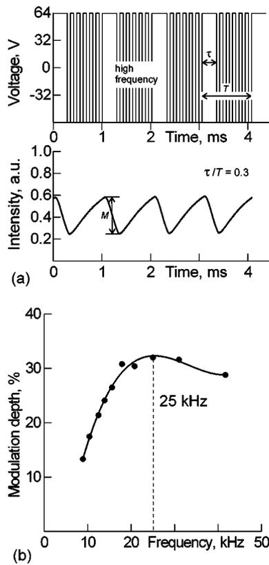
FIG. 6. Influence of the high-frequency component on the modulation depth: (a) shape of the control voltage (top) and electrooptical response (bottom); (b) dependency of the modulation depth vs the high-frequency value.
