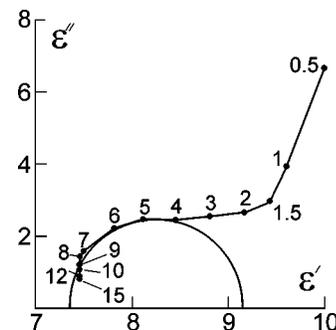
FIG. 5. Cole-Cole diagram for LC1001. The numbers beside the labels are ac voltage frequencies.
