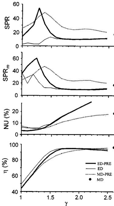
Fig. 5. Performance curves of the various encoding algorithms as a function of  $\gamma$  for the on-axis test function.<sup>25</sup> For ED-PRE the specific curve shown for NU is for  $\chi = 0.9$ , for SPR is for  $\chi = 0.6$ , and for  $SPR_m$  is for  $\chi = 0.7$ . These curves achieve the best performance for ED-PRE as reported in Table 1.
