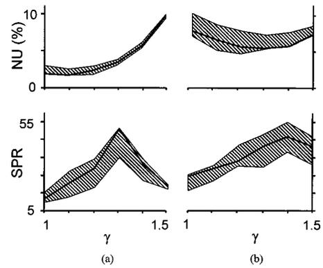
Fig. 7. Statistical variations of the fidelity metrics of (a) ED-PRE and (b) MD-PRE for an ensemble of encodings of the on-axis function. Shaded regions are bounded by the maximum and minimum values found for 21 random trials of each encoding algorithm. The respective curves from Fig. 5 are reproduced for comparison.
