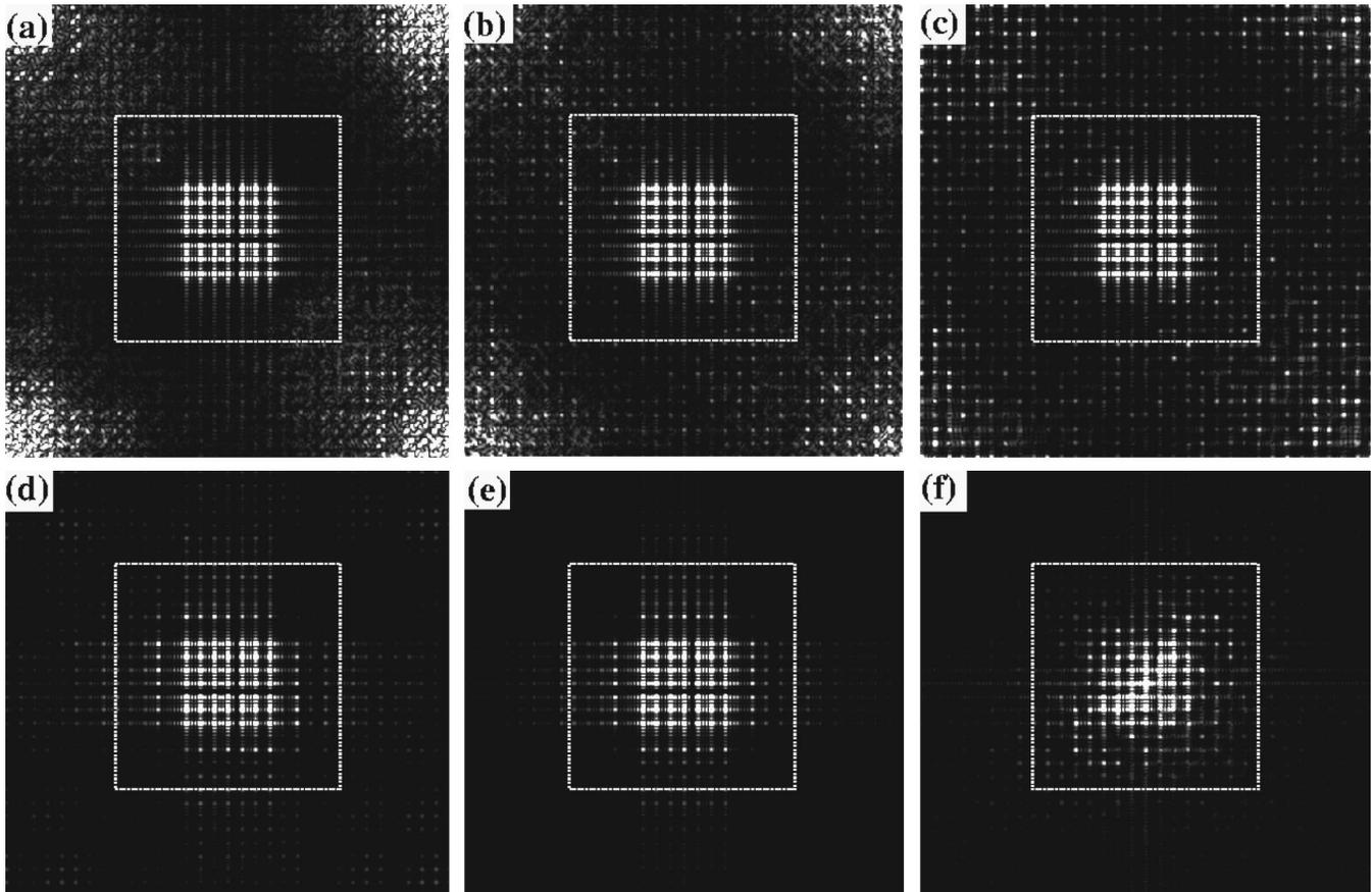
Fig. 3. On-axis diffraction patterns for encoding by (a)–(d) and (f) ED and (e) MDE. The value of  $\gamma$  used for ED is (a) 1.0, (b) 1.2, (c) 1.3, (d) 1.6, and (f) 5.5. The dotted square encloses the area used to calculate  $\text{SPR}_m$ . The gray-scale intensities are scaled so that full white corresponds to 3% of the average peak intensities of the 49 desired spots.
