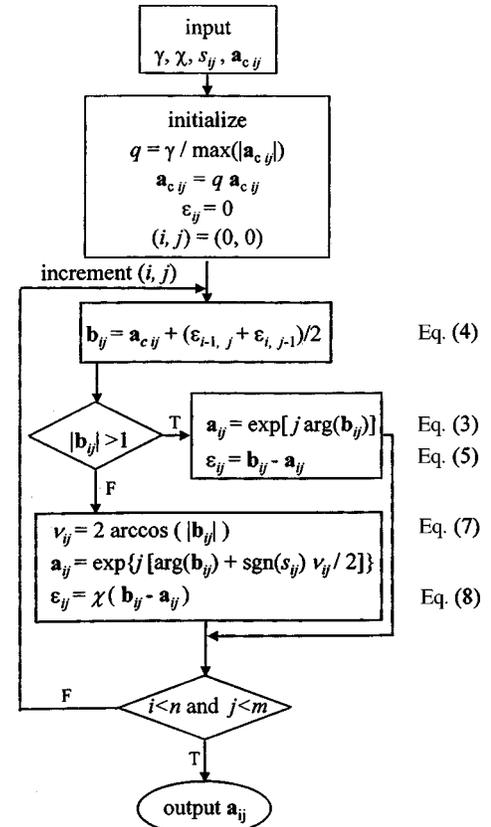
Fig. 2. Flow chart for the ED-PRE algorithm.
