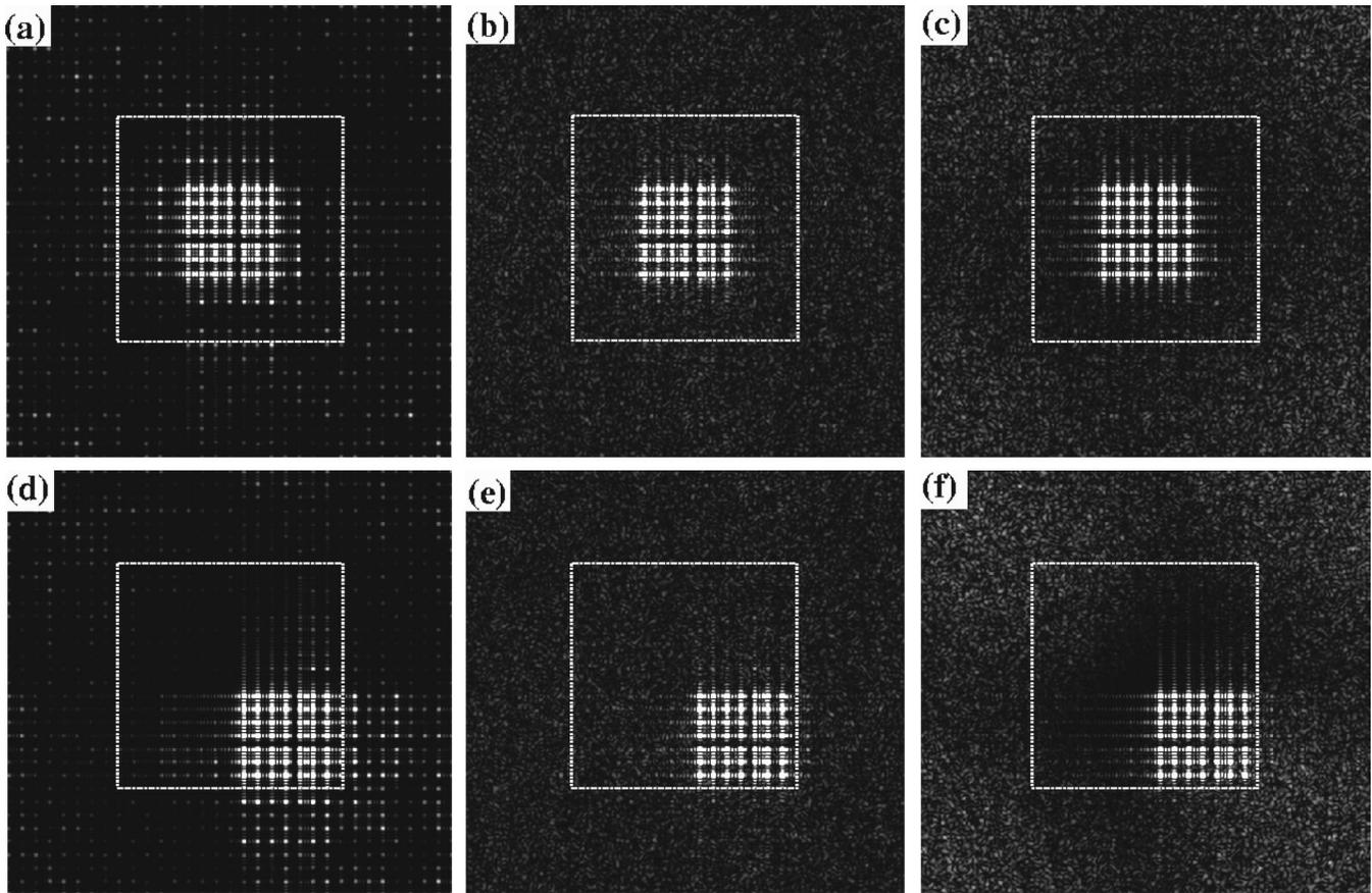
Fig. 4. (a)–(c) On-axis and (d)–(f) off-axis diffraction patterns for the maximum SPR design by (a) ED,  $\gamma = 1.5$ ; (b) MD–PRE,  $\gamma = 1.4$ ; (c) ED–PRE,  $\gamma = 1.3$ ,  $\chi = 0.6$ ; (d) ED,  $\gamma = 1.5$ ; (e) MD–PRE,  $\gamma = 1.4$ ; (f) ED–PRE,  $\gamma = 1.3$ ,  $\chi = 1$ . The gray-scale normalization and the dotted square are identical to those used in Fig. 3.
