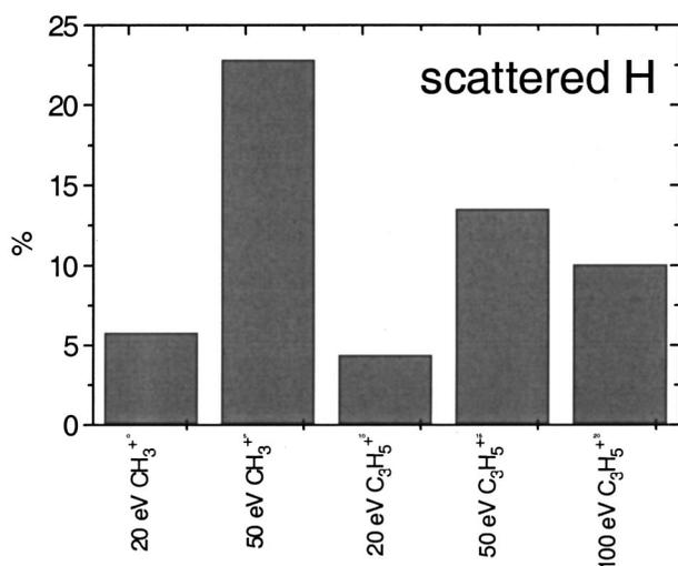
FIG. 7. Illustration of the percentage of hydrogen atoms scattered from the surface after the deposition of CH<sub>3</sub><sup>+</sup> and C<sub>3</sub>H<sub>5</sub><sup>+</sup> (CH<sub>2</sub>-C<sup>+</sup>H-CH<sub>2</sub>) on PS at incident energies of 20, 50, and 100 eV. The results represent the averaged data from 40 trajectories for each incident ion and kinetic energy.
