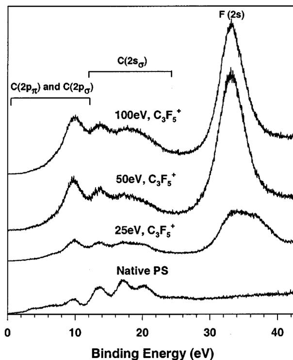
FIG. 2. Valence band XPS of native PS thin film (bottom), and same modified by 25, 50, and 100 eV  $\text{C}_3\text{F}_5^+$  (top).
