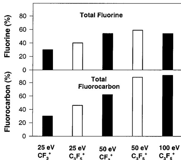
FIG. 4. Percentages of total fluorine (top) and fluorocarbon (bottom) after modification by 25–100 eV  $CF_3^+$  and  $C_3F_5^+$ .
