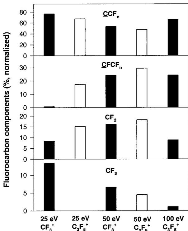
FIG. 5. Percentages of each fluorocarbon component (normalized after removal of the nonfluorinated C(1s) peak component) after modification by 25–100 eV  $\text{CF}_3^+$  and  $\text{C}_3\text{F}_5^+$ .
