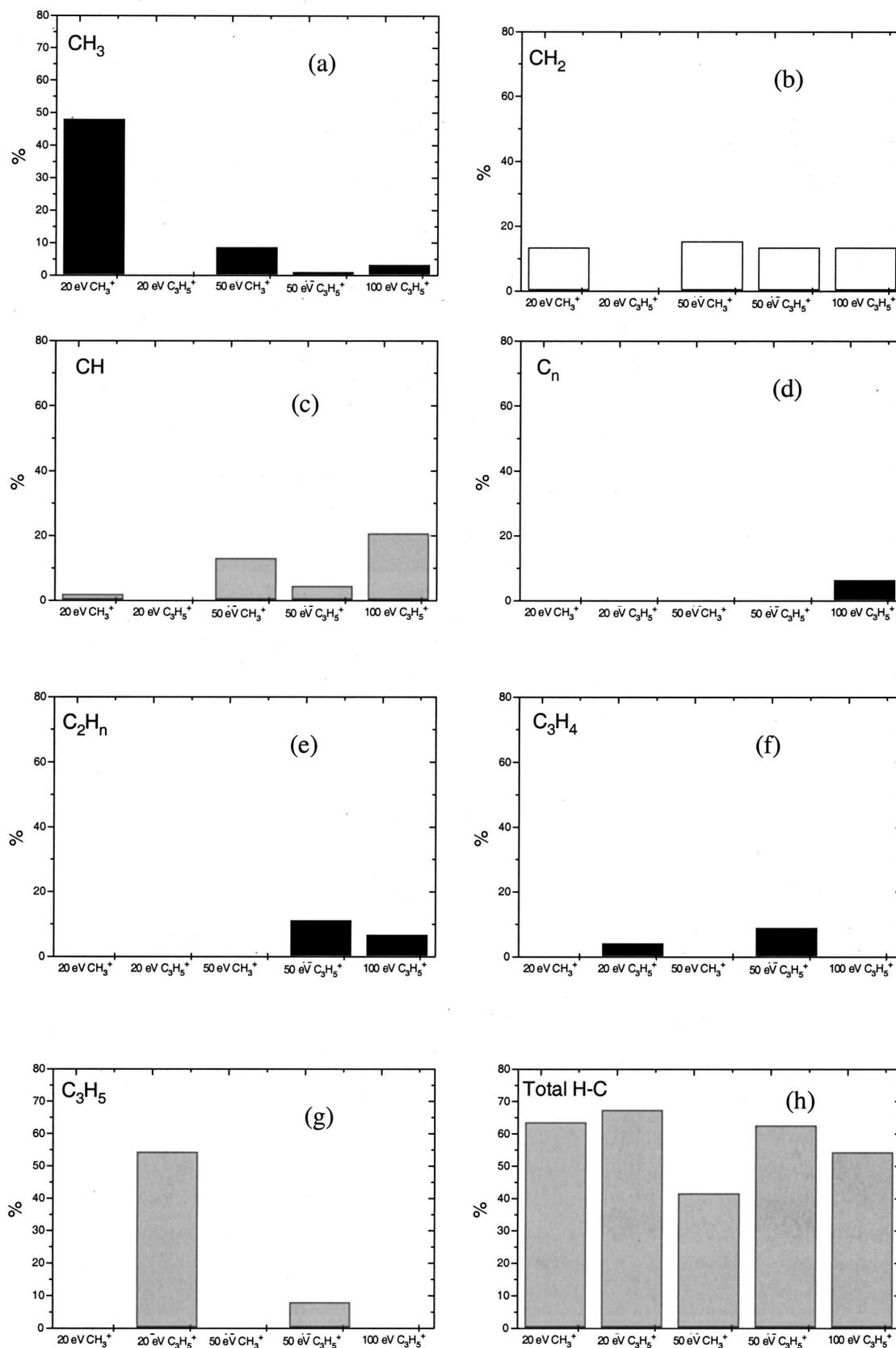
FIG. 6. Summary of the computational results for the deposition of CH<sub>3</sub><sup>+</sup> and C<sub>3</sub>H<sub>5</sub><sup>+</sup> (CH<sub>2</sub>-C<sup>+</sup>H-CH<sub>2</sub>) on PS at incident kinetic energies of 20, 50, and 100 eV, showing the percentage of the indicated product species that remain bonded to or embedded in the PS surface. The results represent the averaged data from 40 trajectories for each incident ion and kinetic energy.
