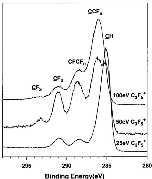
FIG. 1. C(1s) region of XPS of PS thin films modified by 25 (bottom), 50 (middle), and 100 eV  $\text{C}_3\text{F}_5^+$  (top). This and all subsequent spectra recorded at ion fluence equivalent to  $1.5 \times 10^{16}$  F atoms/cm<sup>2</sup>, unless otherwise noted. Components of C(1s) peak are labeled, with detected carbon atom underlined.
