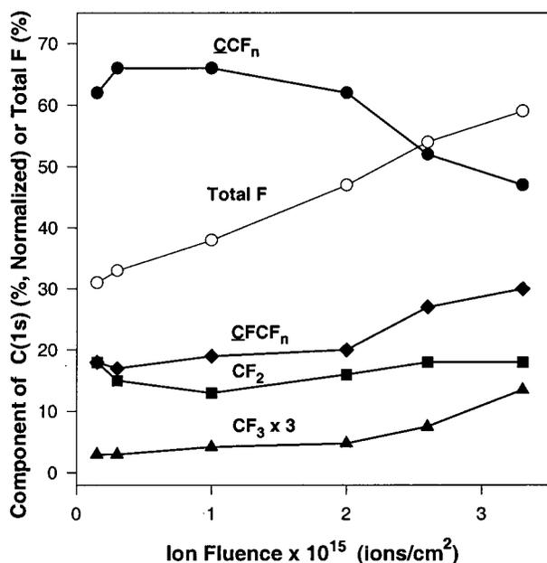
FIG. 3. Total fluorine and individual fluorocarbon component percentages (normalized) on PS following modification with 50 eV  $C_3F_5^+$  ions at fluences ranging from 0.15 to  $3.3 \times 10^{15}$  ions/cm<sup>2</sup>.
