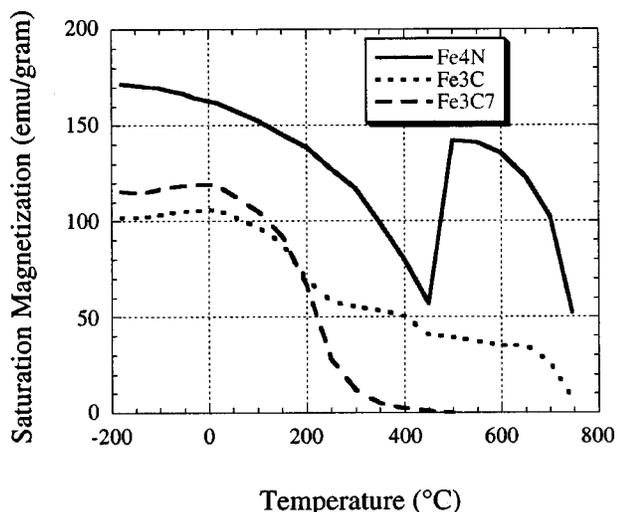
FIG. 4. Saturation magnetization of  $\text{Fe}_3\text{C}$ ,  $\text{Fe}_7\text{C}_3$ , and  $\gamma'$ - $\text{Fe}_4\text{N}$  nanoparticles as a function of temperature.
