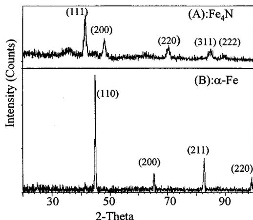
FIG. 2. X-ray diffraction patterns of  $\text{Fe}_4\text{N}$  powders. (A)  $\gamma'$ - $\text{Fe}_4\text{N}$  (before annealing). (B)  $\alpha$ -Fe (after annealing,  $\gamma'$ - $\text{Fe}_4\text{N}$  has decomposed into  $\alpha$ -Fe).
