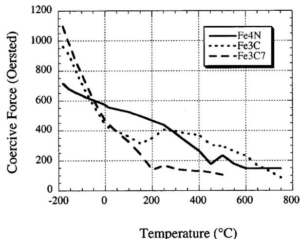
FIG. 5. Coercive force of  $\text{Fe}_3\text{C}$ ,  $\text{Fe}_7\text{C}_3$ , and  $\gamma'$ - $\text{Fe}_4\text{N}$  nanoparticles as a function of temperature.
