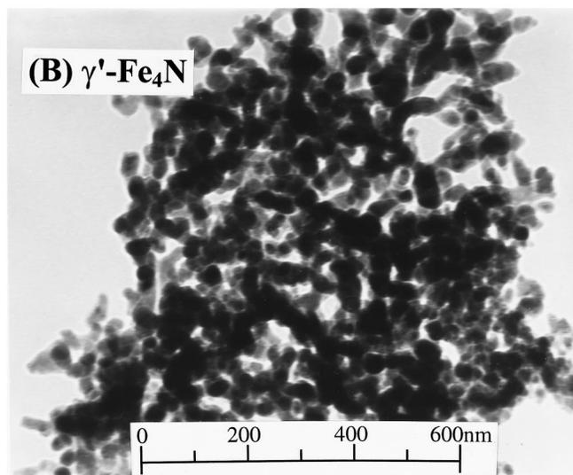
FIG. 3. TEM image of nanoparticles (A)  $\text{Fe}_3\text{C}$ , (B)  $\gamma'$ - $\text{Fe}_4\text{N}$ .
