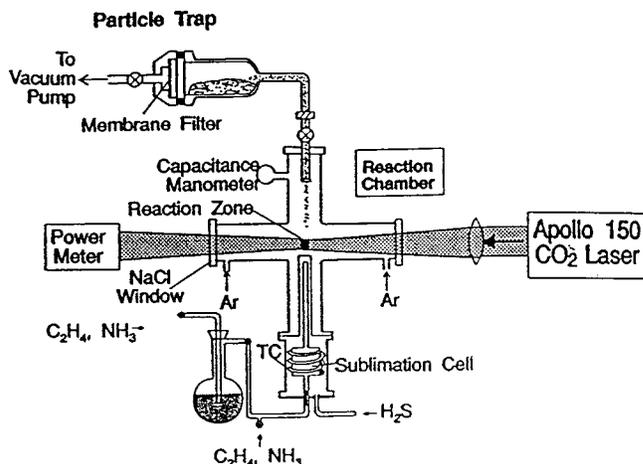
FIG. 1. Schematic drawing of laser pyrolysis system.
