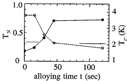
FIG. 4. The transmission coefficient  $T_N$  given by  $(1+Z^2)^{-1}$  and the critical temperature  $T_c$  of Sn near the interface as a function of alloying time. Lines are free interpolations to guide the eye.
