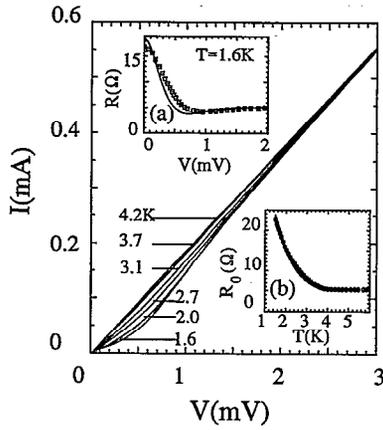
FIG. 1.  $I$ - $V$  characteristics of an unalloyed Sn/GaAs contact at a number of temperatures. The inset (a) shows the differential resistance  $R$  vs bias voltage, measured at 1.6 K. The inset (b) shows the differential resistance  $R_0$  at zero bias vs temperature. In the insets the points represent experimental data and the curves theoretical results calculated using the BTK model.
