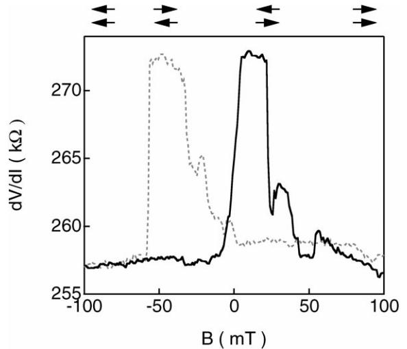
Fig. 2. Two-terminal differential resistance as a function of magnetic field for a Co-contacted MWNT. The magnetic field is directed parallel to the substrate, and the temperature is 4.2 K. The solid (dashed) trace corresponds to the positive (negative) sweep direction. The magnetization direction of the left and right contacts is represented by the arrows at the top of the figure.
