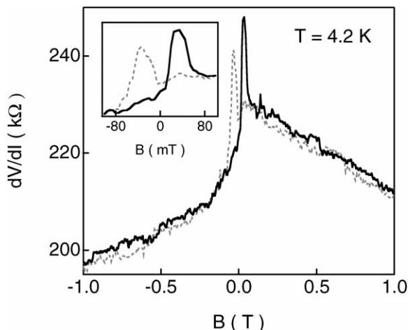
Fig. 3. Magnetoresistance of a second Co-contacted MWNT, showing the behaviour at high-magnetic field. The solid (dashed) line corresponds to the positive (negative) sweep direction. The inset details the region near zero field.
