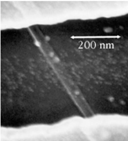
Fig. 1. Electron beam micrograph of a typical Co-contacted multi-walled nanotube. The Co contacts lie on top of the nanotube. The diameter of this particular nanotube is 40 nm; nanotube diameters ranged between 10 and 50 nm.
