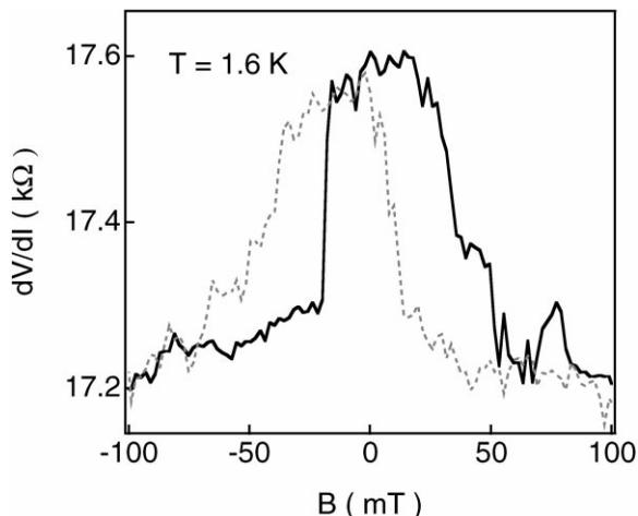
Fig. 4. Magnetoresistance of a MWNT contacted with two different ferromagnetic materials: Co and NiFe. The device is fabricated using a shadow evaporation technique. The solid (dashed) line corresponds to the positive (negative) sweep direction.
