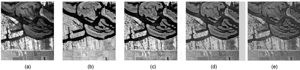
**Fig. 9** Image fusion with remote sensing images ( $512 \times 512$  pixels): (a) image A (IR), (b) image B (low light), (c) image fused by iterative *aDWTi*, (d) image fused by Laplacian pyramid, and (e) image fused by regular DWT.
