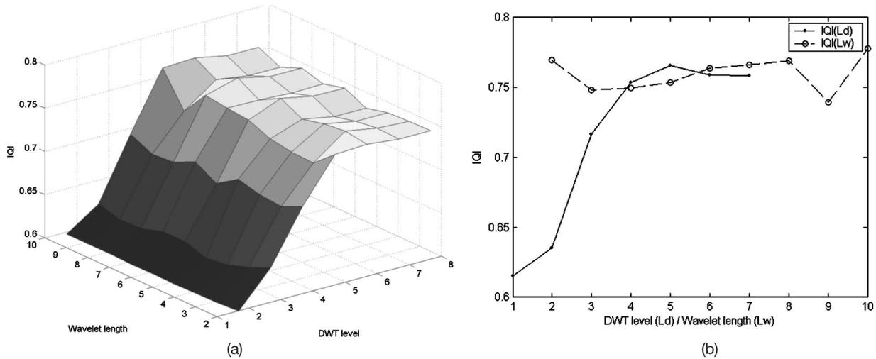
**Fig. 5** IQI distribution with varying parameters of DWT level ( $L_d$ ) and wavelet length ( $L_w$ ) while fusing the medical image pair for (a) distribution of IQI ( $L_d, L_w$ ) and (b) distribution of IQI ( $L_d$ ) and IQI ( $L_w$ )—two slices of (a) at  $L_w=4$  and  $L_d=4$ , respectively. (b) Clearly shows an almost increasing function of IQI ( $L_d$ ), while IQI ( $L_w$ ) is locally fluctuating.
