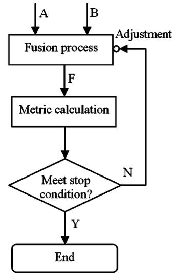
**Fig. 3** Diagram of a general iterative back-propagation fusion process: A and B are input images and F is the fused image.
