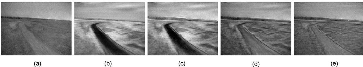
**Fig. 10** Image fusion with the image pair NVESD10 ( $531 \times 401$  pixels) from NV-I1: (a) image A (II), (b) image B (IR), (c) image fused by iterative *aDWTi* (IQI=0.817), (d) image fused by Laplacian pyramid (IQI=0.716), and (e) image fused by regular DWT (IQI=0.565).
