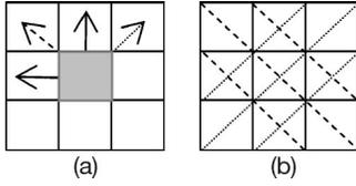
**Fig. 1** Illustration of SF calculation where each small square denotes a pixel: (a) four-directional SFs with arrows pointed to the gradient directions and (b) two diagonal directions; where the dashed lines stand for main diagonal directions and the dotted lines represent secondary diagonal directions.
