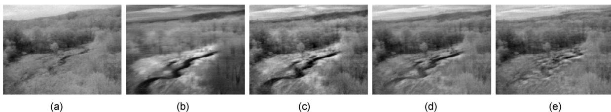
**Fig. 11** Image fusion with the image pair NVESD11 ( $531 \times 401$  pixels) from NV-I1: (a) image A (II), (b) image B (IR), (c) image fused by iterative aDWTi (IQI=0.795), (d) image fused by Laplacian pyramid (IQI=0.768), and (e) image fused by regular DWT (IQI=0.602).
