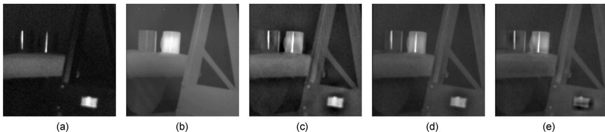
**Fig. 13** Image fusion with the image pair Lab15 ( $220 \times 220$  pixels) from NV-I2: (a) image A (near IR), (b) image B (IR), (c) image fused by iterative *aDWTi* (IQI=0.852), (d) image fused by Laplacian pyramid (IQI=0.757), and (e) image fused by regular DWT (IQI=0.596).
