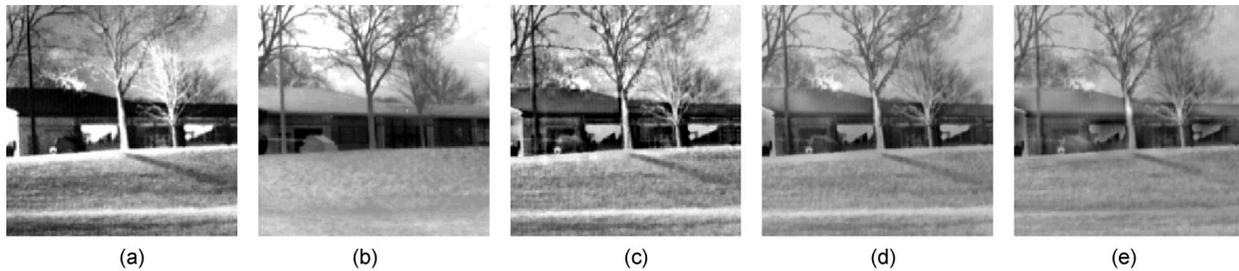
**Fig. 12** Image fusion with the image pair Lab09 ( $220 \times 220$  pixels) from NV-I2: (a) Image a (near IR), (b) image B (IR), (c) image fused by iterative *aDWTi* (IQI=0.756), (d) image fused by Laplacian pyramid (IQI=0.708), and (e) image fused by regular DWT (IQI=0.543).
