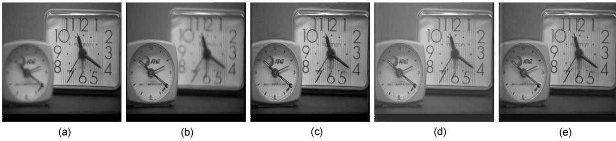
**Fig. 7** Image fusion with off-focus images ( $512 \times 512$  pixels): (a) input image A, (b) input image B, (c) image fused by iterative *aDWTi*, (d) image fused by Laplacian pyramid, and (e) image fused by regular DWT.
