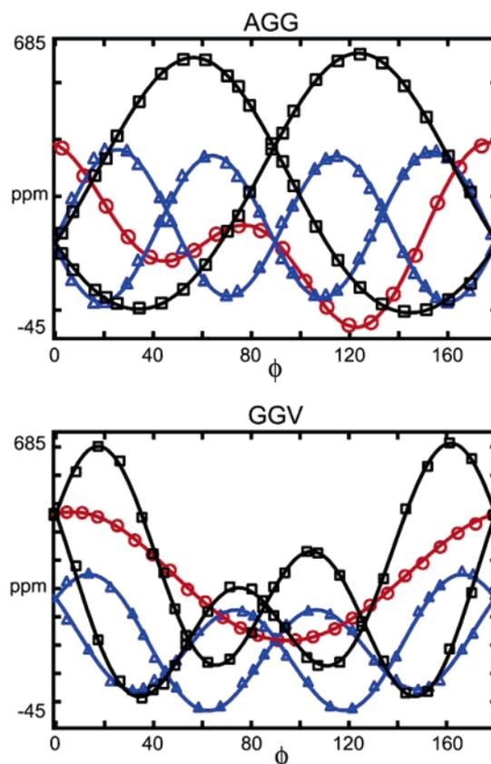
**Figure 2.**  $^{17}\text{O}$  NMR frequencies as a function of crystal orientation for A\*GG and G\*GV. Frequencies for symmetry-related pairs are shown for crystal rotations about the  $a$  (squares),  $b$  (circles), and  $c^*$  (triangles) axes.
