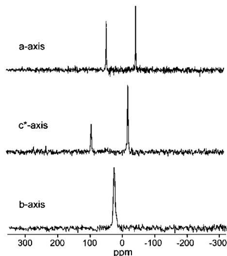
**Figure 1.** <sup>17</sup>O spectra (~1k transients) from a 1 mg GGV crystal. On the basis of the enrichment level (17%), the spectra correspond to detection of ~0.4 μm.
