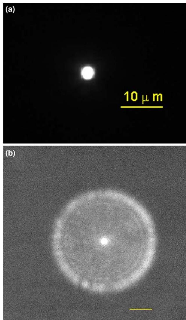
**Fig. 2** Fluorescent imaging of focused and defocused particles with a 60× water immersion lens (numerical aperture-1.2). **a** A 2 μm bead which is in focus. **b** The same bead is placed 30 μm out of focus
