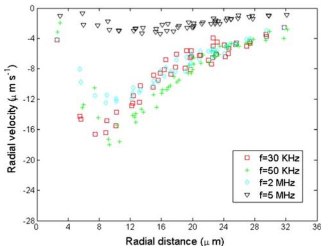
**Fig. 9** Velocimetry results as a function of frequency. All measurements were performed at  $V = 4 V_{pp}$  and  $P = 20 \text{ mW}$
