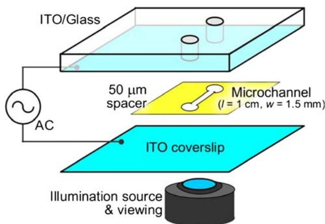
**Fig. 3** An illustration of the microchannel used for the microvortex experiments. The bottom electrode is  $\sim 170 \mu\text{m}$  thick to allow access to a high numerical aperture lens. The length of the microchannel is approximately 1 cm and the width is 1.5 mm. The ports on the top electrode allow fluid to enter the microchannel
