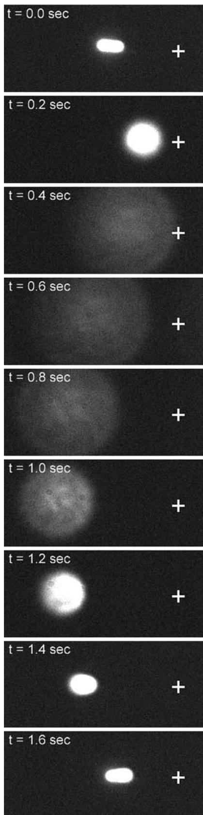
◀ **Fig. 5** A large tracer particle (2  $\mu\text{m}$ ) is caught within the vortex and follows the fluid streamlines with periodic motion. The particle initially moves towards the illumination center (denoted by '+'), goes out of focus as it moves away, and moves towards the focused laser spot again as it comes back into focus
