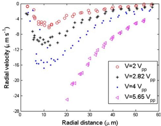
**Fig. 7**  $\mu$ -PIV analysis of the velocity field for vortex flow near the electrode surface.  $V_{pp}$  represents the applied peak-to-peak AC bias. All measurements were performed at  $f = 100$  kHz and  $P = 20$  mW
