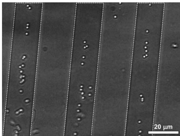
**Fig. 10** Latex particles experiencing negative DEP in the absence of laser heating at  $f = 3 \text{ MHz}$  and  $V = 9 V_{pp}$ . The dotted rectangles indicate the location of the interdigitated ITO electrode strips. Notice that the particles are trapped above the electrodes as illustrated in Fig. 1
