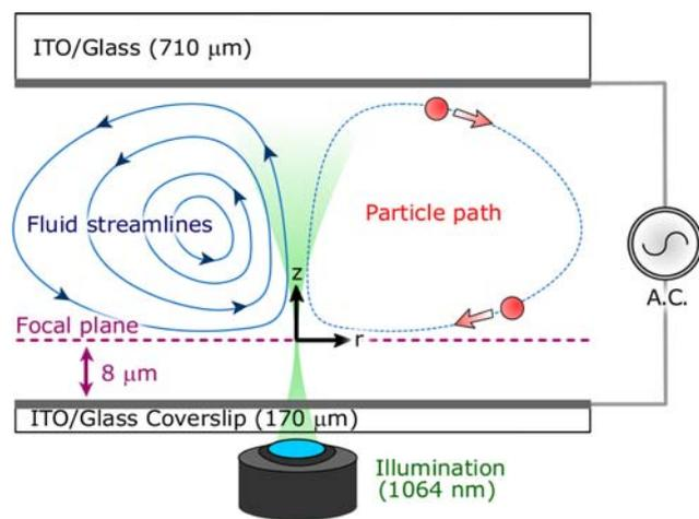
**Fig. 4** An illustration showing location of the measurement plane for flow visualization and  $\mu$ PIV experiments. Note that the measurement plane, focal plane and plane of laser focus are synonymous
