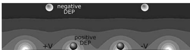
**Fig. 1** Interdigitated electrodes for dielectrophoresis. The *grayscale* contour represents the electric field, with non-uniform regions at the electrode edges. Particles experiencing positive DEP are attracted to these non-uniform regions. Particles experiencing negative DEP are repelled from these regions and, if the height chamber is relatively low, they are located above the middle of the electrode digits
