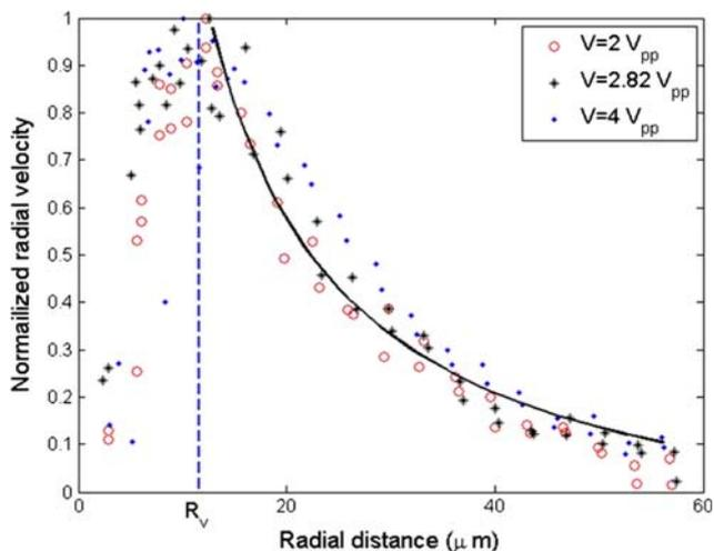
**Fig. 8** Normalized plot for radial velocities. The *curve* represents best fit sink type behavior, i.e.  $v_r = a/r + b$
