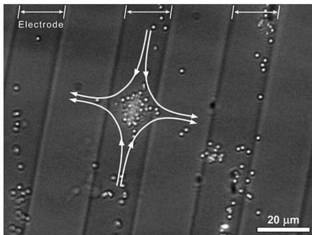
**Fig. 11** Illustrated behavior of the OEMV for interdigitated electrodes with the laser focal point located in the middle of an electrode digit. Electrodes are labeled with arrows at the top of the figure. The direction of the fluid flow is depicted with curved arrows with the laser focus occurring in the middle of the vortex. Particles are pushed with the fluid towards the illumination spot and a few are ejected perpendicular to the edge of the electrode
