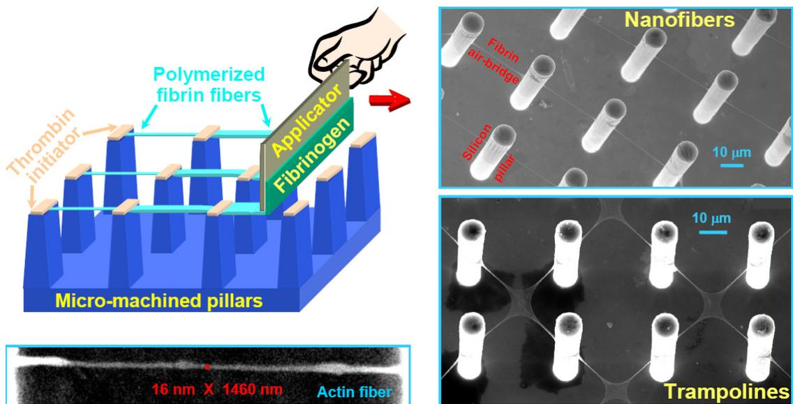
Figure 1. Hand brush on method of directed self-assembly of nanofiber air-bridges and trampolines. The particular reaction shown is for thrombin enzyme-initiated polymerization of fibrin from fibrinogen precursor.
