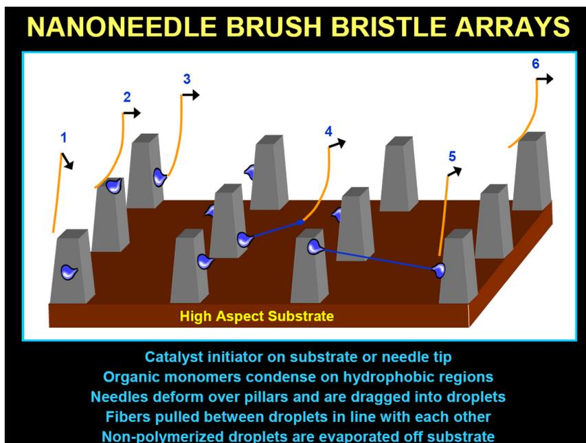
Figure 4. SmartBrush: A proposed process of using arrays of individually actuated nanoneedles to pattern rather arbitrary point-to-point nanofibers air-bridges in a 3D addressing space.
