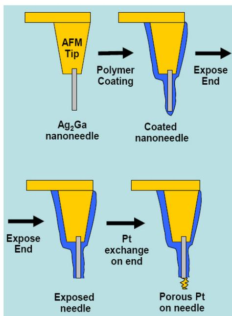
Figure 3. Process flow for templated fabrication of an electrochemical nanoelectrode.
