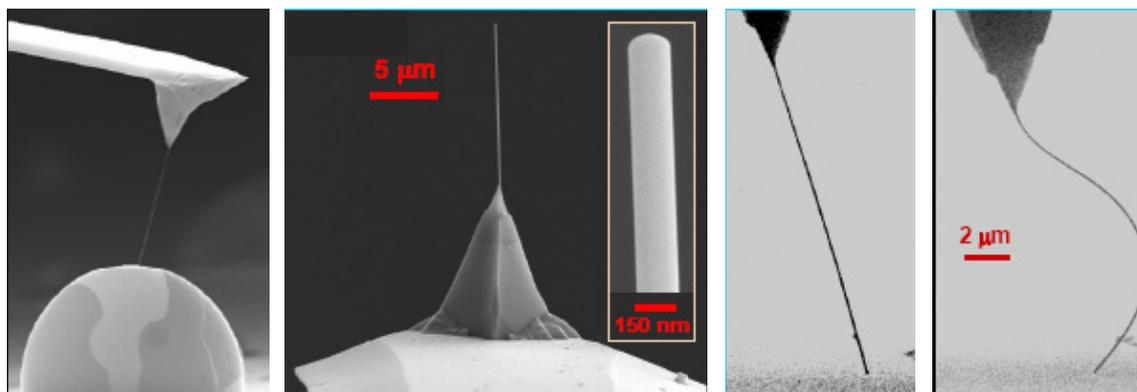
Figure 2. Growth and flexibility of an individual metal alloy nanoneedle. In under 5 min the  $\text{Ag}_2\text{Ga}$  needle was directed to grow on the end of a Ag-coated AFM tip after it was dipped into a 25 °C melt of gallium.
