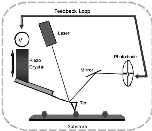
**Figure 1: AFM setup**
