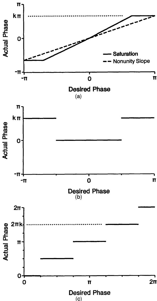
Fig. 1. Various systematic phase errors: (a) two continuous mappings for which the actual phase has less than a  $2\pi$  range of modulation, (b) binary phase-only mapping in which the range of phase modulation is not necessarily  $\pi$ , (c) mapping in which the actual phase is quantized into  $m$  levels [in which Eq. (1) gives the relationship between  $k$  and  $m$ ].
