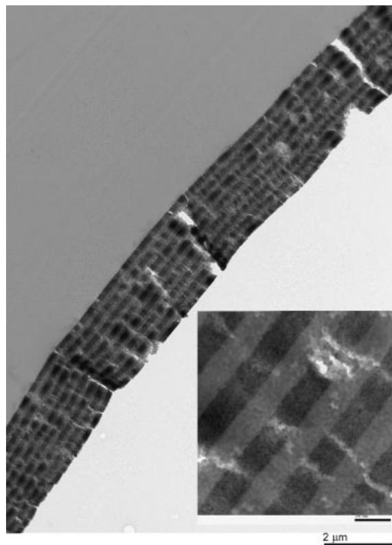
**Figure 3.** Cross-section TEM image of the nanocomposite infrared filter, where the dark section is the TiO<sub>2</sub> and the lighter section is SiO<sub>2</sub>. Inset is a closer view (approximately 10 $\times$  magnification) showing the nanoparticles embedded in the polymer matrix.
