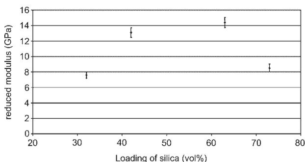
**Figure 1.** Reduced modulus of elasticity of a nanocomposite TMPTA film at different SiO<sub>2</sub> packing densities, exhibiting a maximum at about 60 vol % nanoparticle loading.
