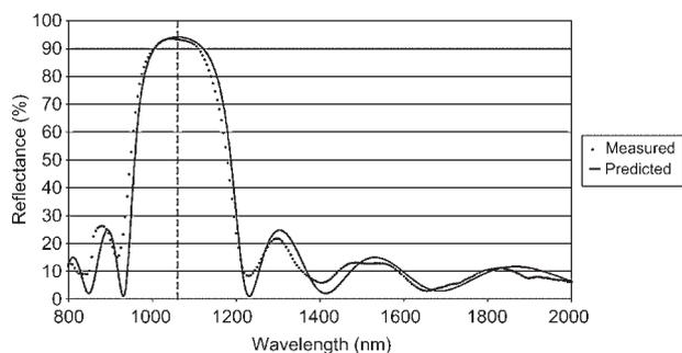
**Figure 2.** Measured and predicted reflectance spectrum of the 15 layer stack.
