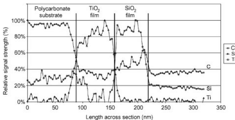
**Figure 4.** Elemental mapping of a two-layer stack conducted using three elements: titanium, silicon and carbon. Each element is mapped by the ratio of the signal strength (counts) to the maximum signal for that element expressed as a percent.
