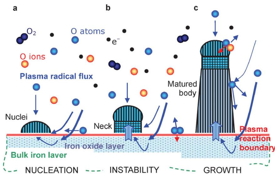
**Figure 5.** Schematic illustration of the growth mechanism of the metal oxide nanowires from bulk material when exposed to highly dissociated oxygen plasma. Three main stages of nanowire growth are represented: a) nucleation, b) instability, c) growth.
