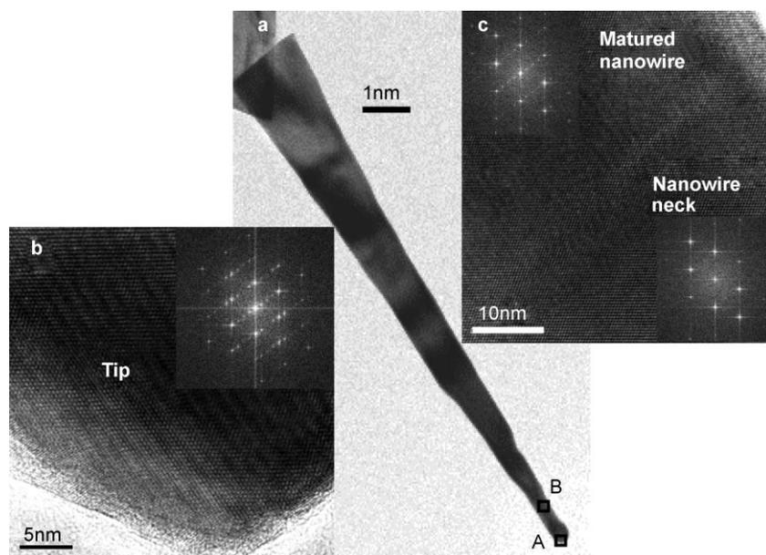
**Figure 4.** a) High-magnification TEM images of nanowires with HREM image and its FFT image showing oxygen-vacancy ordering in  $\alpha - \text{Fe}_2\text{O}_3 \frac{1}{4}(\bar{1} 12)$  plane of b) the nanowire tip and c) the matured nanowire, but not on the nanowire neck area.
