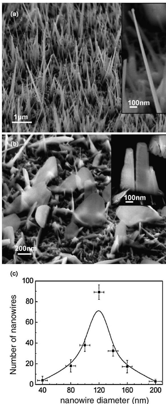
**Figure 1.** SEM images of iron oxide nanostructures grown on Fe bulk material during oxygen plasma treatment at 100 Pa. The entire surface is covered with a large array of  $\alpha\text{-Fe}_2\text{O}_3$  a) nanowires or b) nanobelts. The average diameter of the nanowires is 120 nm. c) The distribution curve of nanowire diameter (a) within a  $100\text{-}\mu\text{m}^2$  area indicates spontaneous nucleation of nanowires.
