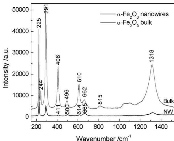
**Figure 2.** Raman spectroscopy reveals the  $\alpha\text{-Fe}_2\text{O}_3$  oxide layer, nanowires, and nanobelts on bulk Fe surface prepared by oxygen plasma treatment.
