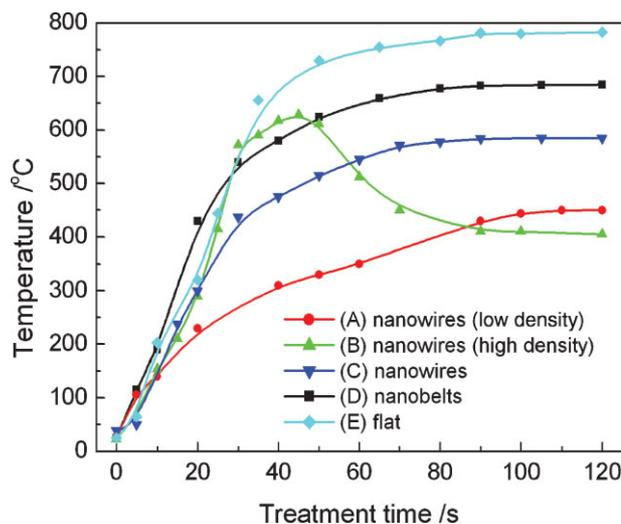
**Figure 3.** The surface temperature of the iron oxide samples during plasma treatment and synthesis of nanowires, nanobelts, or flat thin films.
