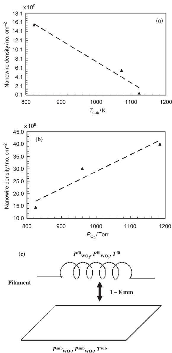
**Figure 3.** a) Experimental data showing the nanowire density obtained as a function of substrate temperature. b) Experimental data showing the effect of partial pressure of oxygen on the nanowire density at lower substrate temperature (823 K). c) Schematic image describing the equilibrium parameters at the filament and at the substrate used for estimating the imposed gas-phase supersaturation at the substrate.
