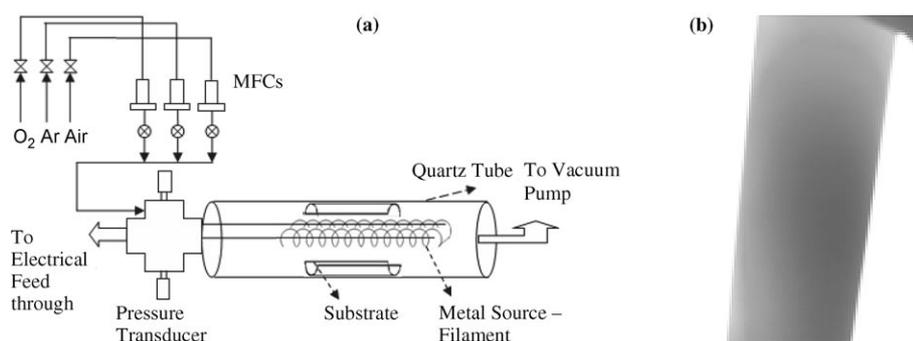
**Figure 6.** a) Schematic image of the hot-filament CVD reactor using tungsten filaments. MFC: mass-flow controller. b) Optical image showing the uniform coating of the tungsten oxide nanowire arrays on a quartz substrate.
