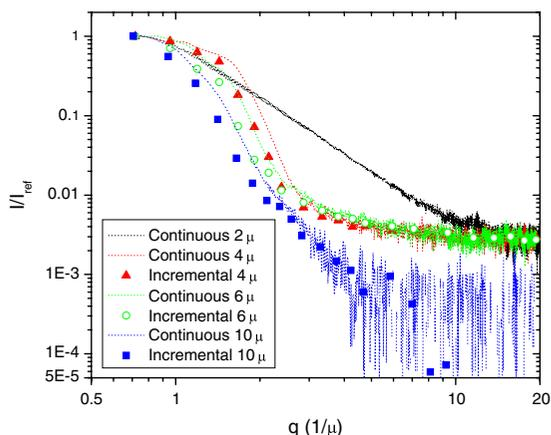
**Fig. 8** Small angle static light scattering measurements for aggregates of 2, 4, 6, 10  $\mu\text{m}$   $\text{WO}_3$  single nanowires. Linear fits (not shown) for incremental data points between  $\theta = 7^\circ$ – $10^\circ$ ,  $\theta = 6^\circ$ – $9^\circ$ , and  $\theta = 5^\circ$ – $8^\circ$  give  $Slope = -7.48$ ,  $Slope = -6.63$ , and  $Slope = -6.28$  for 4, 6, and 10  $\mu\text{m}$  nanowires, respectively
