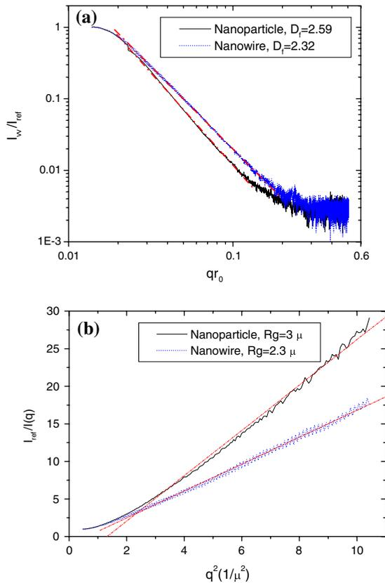
**Fig. 5** (a). Determination of fractal dimension using small angle static light scattering. Aggregates of  $WO_3$  irregular nanoparticles (lower curve) and uneven nanowires (upper curve) in EtOH. (b).  $R_g$  for aggregates of irregular  $WO_3$  nanoparticles and uneven nanowires in EtOH. Linear fits (dash-dot) are for data points between  $\theta = 6^\circ-14^\circ$
