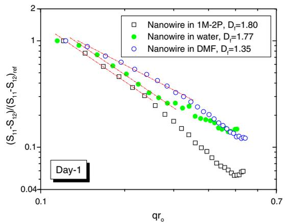
**Fig. 6** Determination of fractal dimension using elliptically polarized light scattering. Aggregates of  $2 \mu\text{m}$  average length bundled  $WO_3$  nanowires in 1-methoxy-2-propanol (1M-2P), water and N,N-dimethylformamide (DMF) on Day-1. Linear fit is for incremental data points between  $\theta = 25^\circ-50^\circ$ ,  $\theta = 30^\circ-65^\circ$  and  $\theta = 30^\circ-70^\circ$ , respectively
