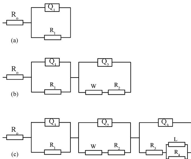
Fig. 6. The equivalent circuits used to fit the impedance data of the zinc electrode polarized at  $E = -1.6$  V (a),  $E = -1.35$  V (b) and  $E = -1.2$  and  $-1.1$  V (c) in 0.1 M  $\text{KClO}_4$ .
