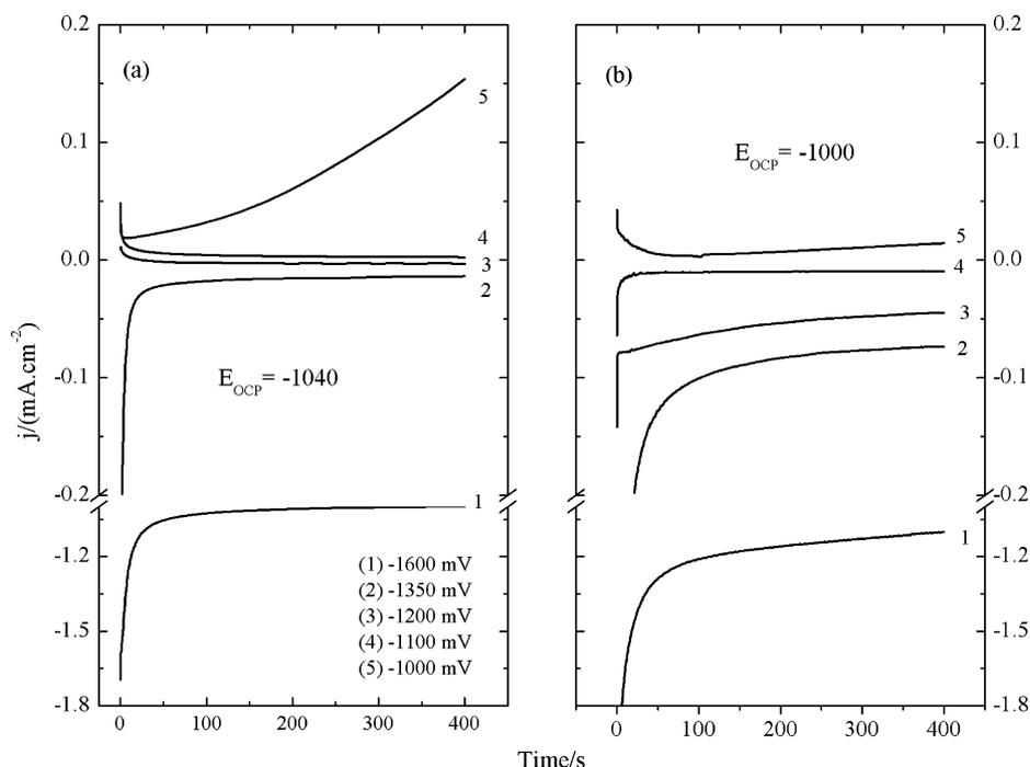
Fig. 4. Chrono-amperometric curves for stationary (a) and  $64 \text{ rad s}^{-1}$  rotating (b) Zn electrode in de-aerated  $0.1 \text{ M KClO}_4$  solution at different electrode potential.
