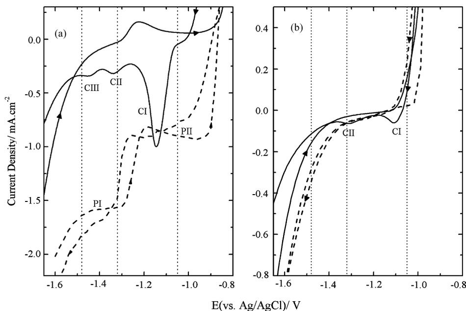
Fig. 1. Cyclic voltammograms for stationary (solid line) and  $64 \text{ rad s}^{-1}$  rotating Zn electrode (dotted lines) in naturally aerated (a) and de-aerated (b) 0.1 M  $\text{KClO}_4$  at scan rate of  $0.5 \text{ mV/s}$ .
