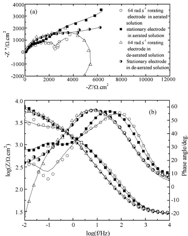
Fig. 9. Nyquist (a) and Bode (b) plots for the zinc electrode at  $-1100\text{ mV}$  in  $0.1\text{ M KClO}_4$  in the frequency range  $10^4\text{--}10^{-2}\text{ Hz}$ . Symbols represent the experimental data and solid lines represent the best fit.
