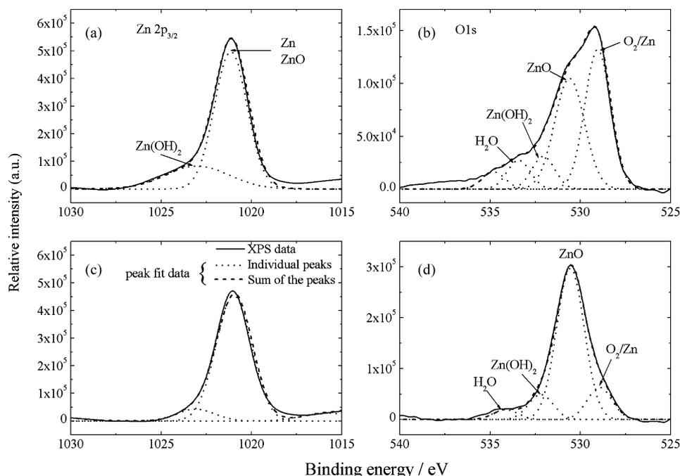
Fig. 2. XPS spectrum of Zn  $2p_{3/2}$  and O 1s for the film formed on zinc electrode polarized from −1.8 to −1.15 V ( $1 \text{ mV s}^{-1}$ ) and hold at −1.15 V for 30 min in naturally aerated (a and b) and de-aerated (c and d) 0.1 M  $\text{KClO}_4$ .
