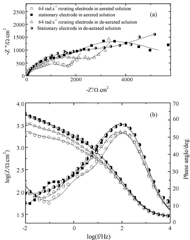
Fig. 8. Nyquist (a) and Bode (b) plots for the zinc electrode at  $-1200\text{ mV}$  in  $0.1\text{ M KClO}_4$  in the frequency range  $10^4\text{--}10^{-2}\text{ Hz}$ . Symbols represent the experimental data and solid lines represent the best fit.
