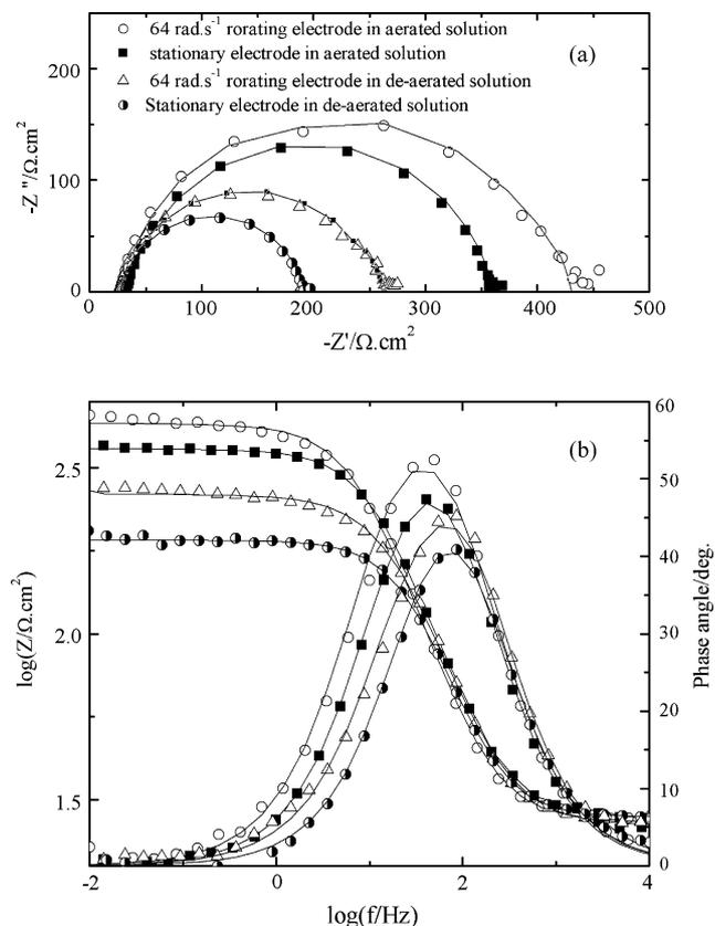
Fig. 5. Nyquist (a) and Bode (b) plots for the zinc electrode at  $-1.6 \text{ V}$  in  $0.1 \text{ M KClO}_4$  in the frequency range  $10^4$ – $10^{-2} \text{ Hz}$ . Symbols represent the experimental data and solid lines represent the best fit.
