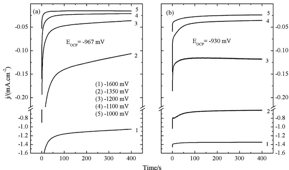
Fig. 3. Chrono-amperometric curves for stationary (a) and  $64 \text{ rad s}^{-1}$  rotating (b) Zn electrode in naturally aerated  $0.1$  M  $\text{KClO}_4$  solution at different electrode potential.
