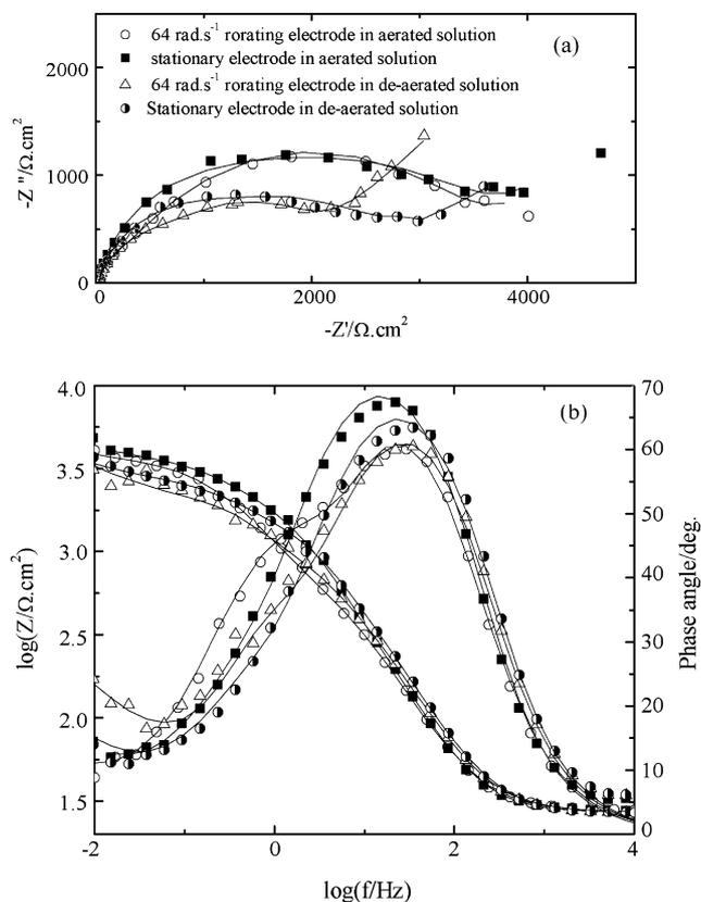
Fig. 7. Nyquist (a) and Bode (b) plots for the zinc electrode at  $-1350\text{ mV}$  in  $0.1\text{ M KClO}_4$  in the frequency range  $10^4\text{--}10^{-2}\text{ Hz}$ . Symbols represent the experimental data and solid lines represent the best fit.
