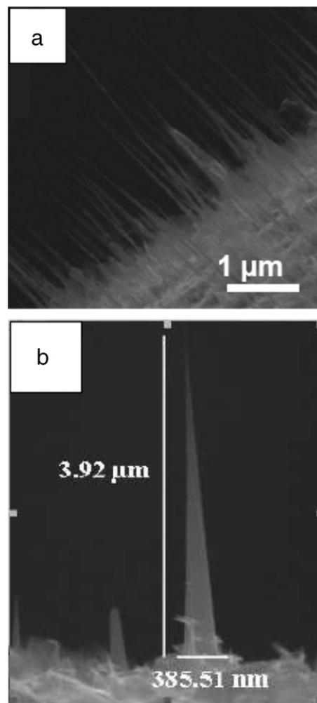
Fig. 2. SEM images of a) CNPs grown on bare platinum substrates, and b) an individual CNP structure.
