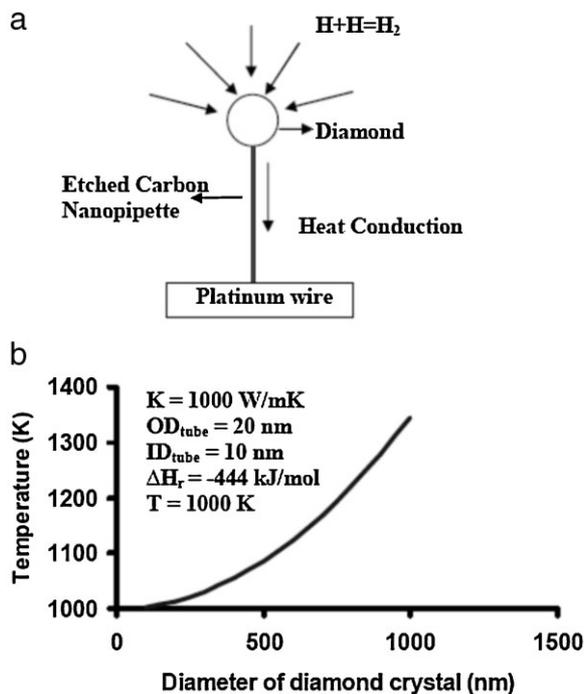
Fig. 4. a) A schematic illustrating the heat runaway scenario for a crystal growing at the tip of a thin CNT. b) A plot showing the estimated temperature rise during diamond growth as a function of diamond crystal size using the parameters indicated.
