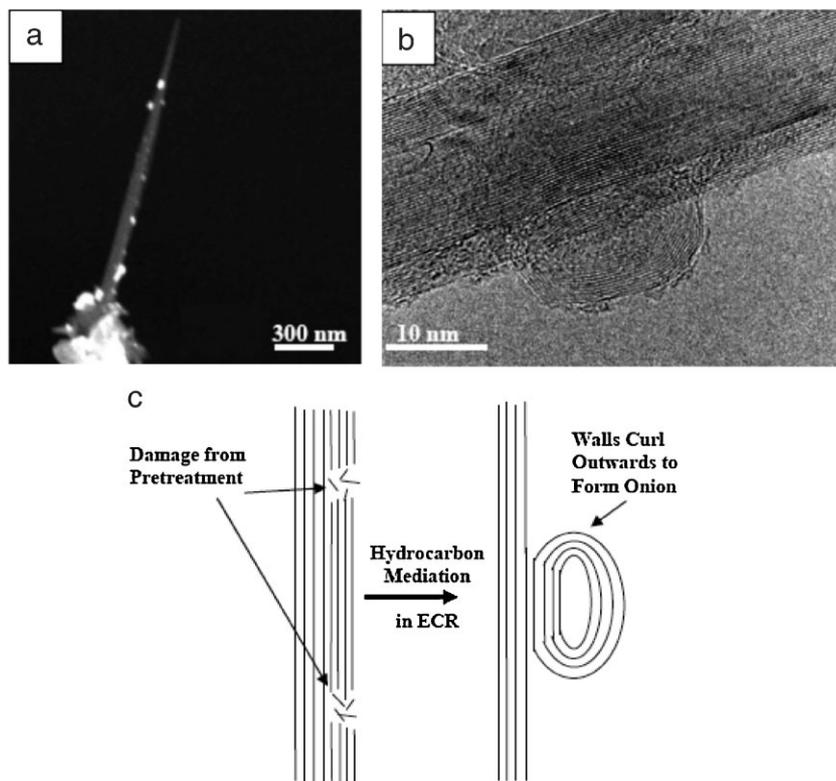
Fig. 6. a) A SEM image showing several bright clusters on the sidewall of CNPs. b) A high resolution image of one of the bright clusters indicating them to be a carbon onion. c) A schematic illustrating the curling mechanism of CNP walls at the damage sites, created during the pretreatment step.
