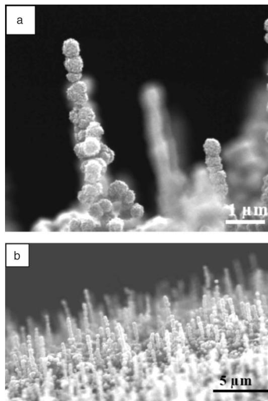
Fig. 8. SEM images showing CNPs treated with boron carbide powder. a) Shows the complete coating of diamond crystals along the length of a CNP clearly depicting the spiral growth of diamond crystals. b) Shows a large array of CNPs coated with diamond crystals.
