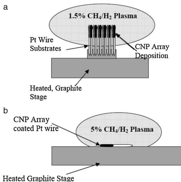
Fig. 1. a) A schematic illustrating the vertical positioning of the platinum wire substrates for the synthesis of CNPs. b) A schematic illustrating the horizontal positioning of the platinum wire substrates coated with CNP arrays for diamond nucleation and growth experiments.
