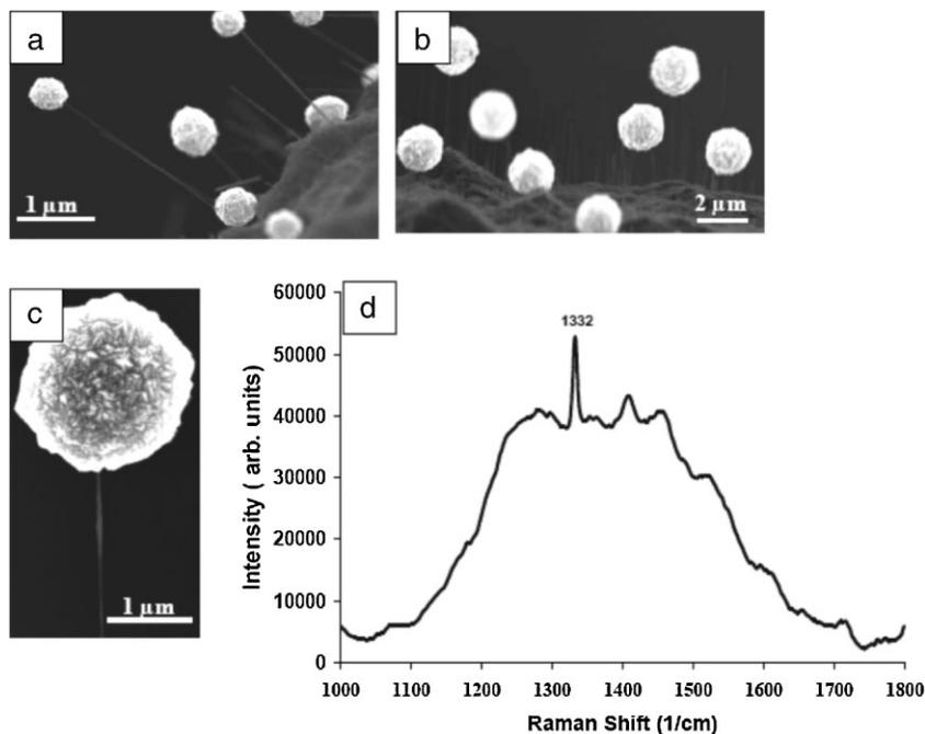
Fig. 3. SEM images of diamond growth on CNPs without pretreatment. a) Selective growth of sub-micrometer-scale crystals on the tips for  $\sim 20$  min. b) Micrometer-scale diamond crystals grown for  $\sim 3$  h. c) A diamond crystal (grown for  $\sim 3$  h) at the tip of the straight carbon nanotube. d) Visible Raman spectra showing a peak at  $1332\text{ cm}^{-1}$  corresponding to the diamond crystals at the tips of the CNPs shown in Fig. 3c.
