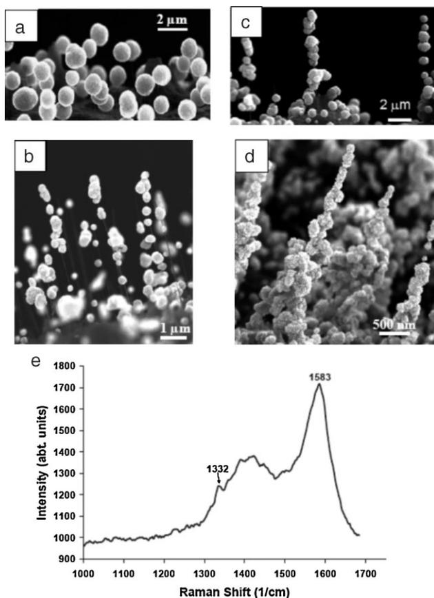
Fig. 7. SEM images showing diamond nucleation and growth on CNPs after pretreatment using the sonic bath dispersions of: a) micrometer-scale diamond powder; and b) sub-micrometer-scale diamond powder. Results of pretreatment using electrophoretic seeding in dispersions of: c) micrometer-scale diamond powder; and d) sub-micrometer-scale diamond powder. e) A UV Raman spectrograph confirming the presence of diamond with a peak at  $1332\text{ cm}^{-1}$ .
