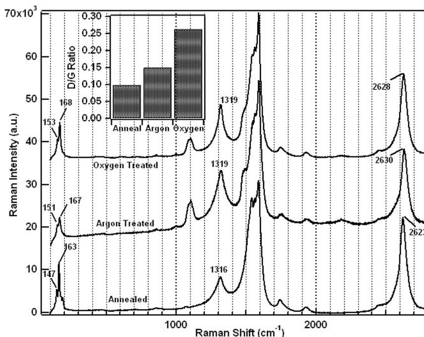
**Figure 1.** Raman spectra at 632 nm laser excitations for pristine, argon plasma treated, and oxygen plasma treated SWNTs, respectively, from bottom to top. The inset shows the histogram of the D band to G band intensity ratio for the three samples.
