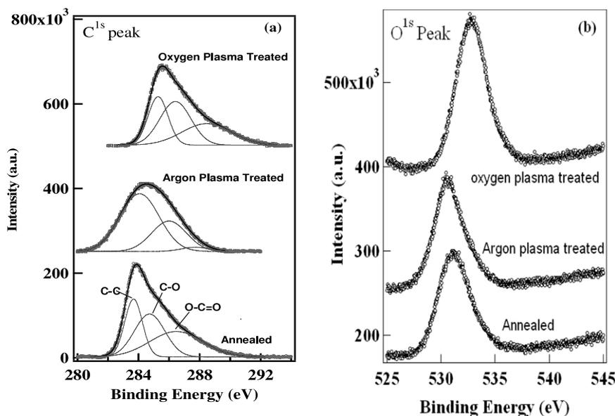
**Figure 2.** XPS data for annealed, argon plasma treated, and oxygen plasma treated SWNTs, respectively, from bottom to top: (a) C 1s peak with best fits to three Gaussians corresponding to C–C, C–O, and O–C=O bonds; (b) O 1s peak.
