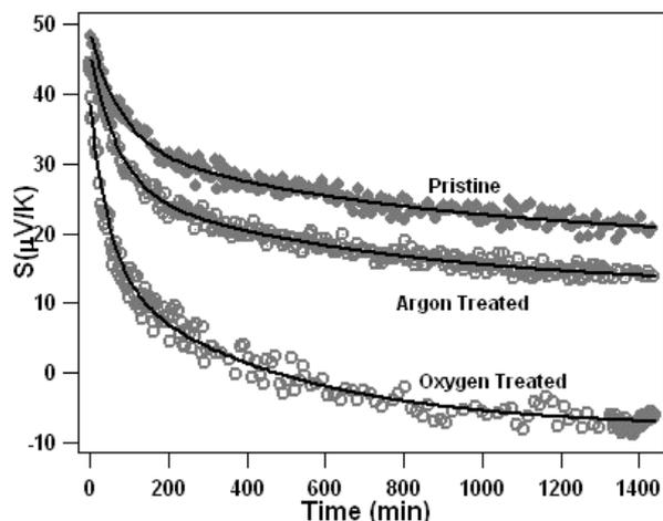
**Figure 4.** Thermopower versus time for three HiPCO samples during desorption of oxygen. Best fits with three exponentials are also shown in solid lines.
