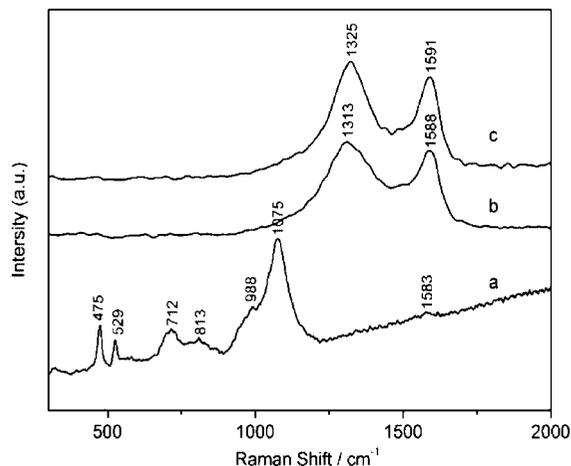
**Figure 2.** Raman spectra for (a) the B<sub>4</sub>C precursor, (b) CDC-600, and (c) CDC-1000. The D:G ratios (based on peak area) are 1.87 and 1.70 for (b) and (c), respectively.
