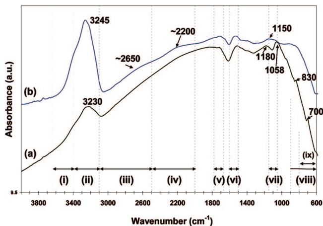
**Figure 4.** FTIR spectra for (a) CDC-600 and (b) CDC-1000. Regions of interest include (i) alcohol O–H stretching; (ii) adsorbed water (O–H stretching); (iii) carboxylic acids O–H stretching; (iv) triple-bond stretching; (v) carbonyl C=O stretching; (vi) aromatic stretching; (vii) alcohol C–O stretching; (viii) C–H out of plane bending; (ix) C–Cl stretch.
