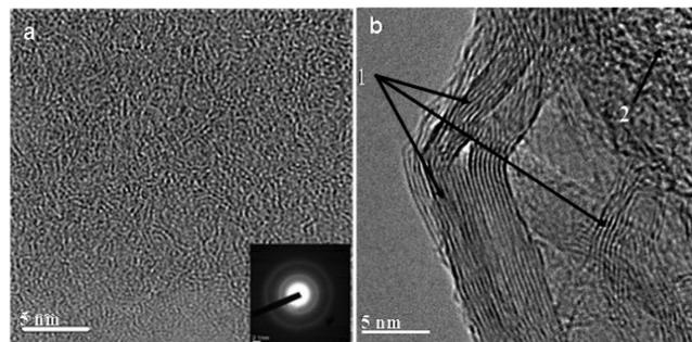
**Figure 1.** (a) HRTEM of CDC-600 shows the carbon structure is noncrystalline but with some texture. The insert SAD indicates the amorphous structure of the CDC. (b) HRTEM of CDC-1000 shows the presence of a mixture of graphitic layers of interplanar distance of 0.34 nm (arrows labeled 1) and a noncrystalline amorphous structure (arrow labeled 2).
