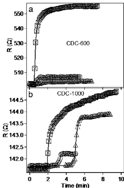
**Figure 5.** Initial resistive response,  $R$ , (at  $P = 10$  torr) to  $\text{NH}_3$  (squares),  $\text{N}_2\text{O}$  (circles) and room air (triangles) versus time of (a) CDC-600 and (b) CDC-1000.
