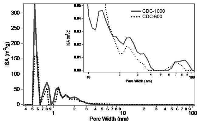
**Figure 3.** Pore size distribution, calculated from N<sub>2</sub> adsorption for CDC-600 (dashed line) and CDC-1000 (solid line) shows preparation conditions alter the pore structure. The inset is a zoom of the macropore and mesopore regions.
