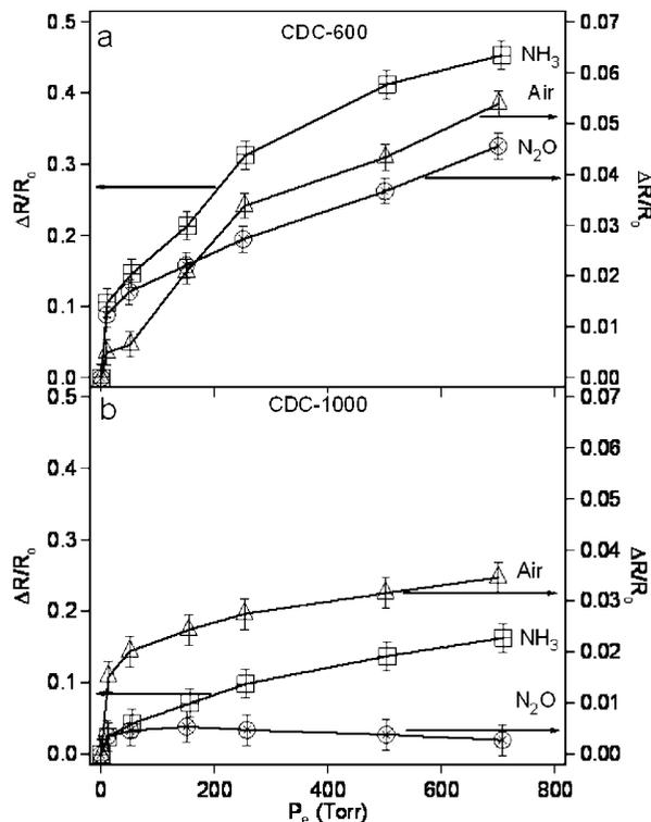
**Figure 6.** Response ( $\Delta R/R_0$ ) versus equilibrium pressure ( $P_e$ ) of  $\text{NH}_3$  (squares),  $\text{N}_2\text{O}$  (circles) and room air (triangles) for (a) CDC-600 and (b) CDC-1000. The gases are plotted on two scales to accommodate large differences in response. Error bars represent one standard deviation of 2–3 measurements on different films of the same material.
