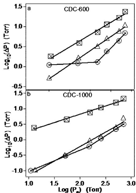
**Figure 7.** Log–log plot of the pressure drop upon gas exposure versus equilibrium pressure ( $P_e$ ) for (a) CDC-600 and (b) CDC-1000 upon exposure to  $\text{NH}_3$  (squares),  $\text{N}_2\text{O}$  (circles) and room air (triangles) over the entire pressure range up to 760 Torr. Pressure drop,  $\Delta P$  is proportional to gas adsorbed, thus the figure is a pseudo-adsorption isotherm (see text).
