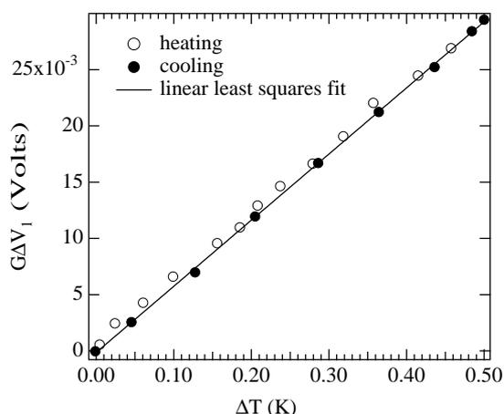
**Figure 4.** A plot of the thermoelectrical response versus the temperature gradient  $\Delta T$ . Open and closed circles represent, respectively, data collected on heating and cooling. The full line is a linear least-squares fit to the data and the slope of this line is the relative sample thermopower.
