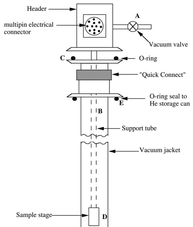
**Figure 2.** A schematic diagram of the thermopower-measurement probe suitable for the temperature range 4–300 K. See the description in the text.
