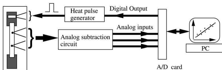
**Figure 3.** A schematic diagram of the system for thermopower measurement by analogue subtraction. See the description in the text.
