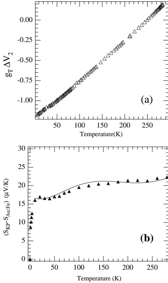
**Figure 5.** (a)  $V_{BA}$  as a function of the sample temperature  $T$ . (b)  $d(V_{BA})/dT$  or  $S_{KP} - S_{Au:Fe}$  versus  $T$ .
