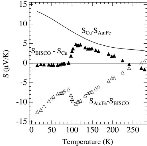
**Figure 7.** The experimentally determined thermoelectrical power of a superconducting sample  $\text{Bi}_2\text{Sr}_2\text{CaCu}_2\text{O}_{7+\delta}$  (BISCO,  $T_c \approx 95$  K).
