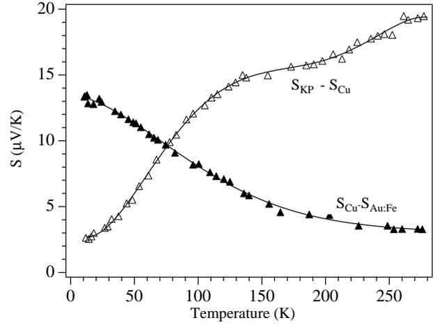
**Figure 6.** Experimentally determined  $S_{KP} - S_{Cu}$  and  $S_{Au:Fe} - S_{Cu}$  as functions of temperature  $T$ . Full lines represent the polynomial fits.
