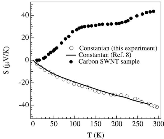
**Figure 8.** Experimental thermoelectrical power data for constantan and single-walled nanotube (SWNT) bundles of carbon. Data for constantan from [8] are shown (full curve) for comparison.
