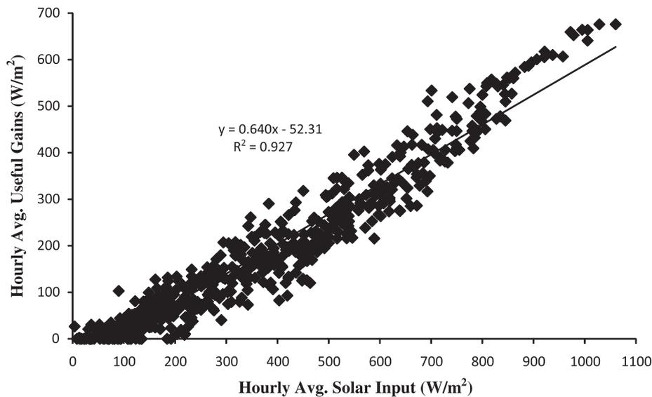
Fig. 8. Plot of hourly average useful gains versus hourly average solar input from 9 am to 5 pm for each day of the heating season.
