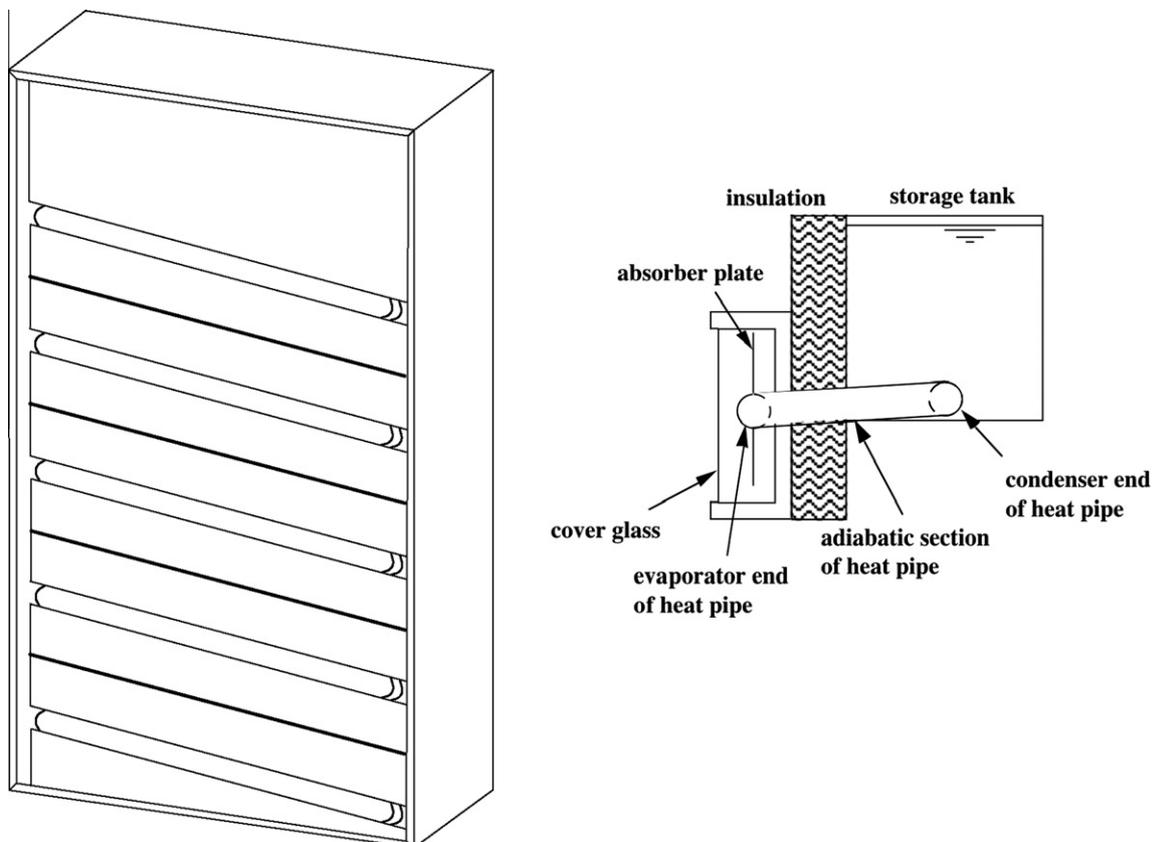
Fig. 4. Left: isometric sketch of the prototype. On the front are the five slanted evaporator sections and absorber plates as seen through the cover glass. The interior components are not visible. Right: 2D schematic of one unit.
