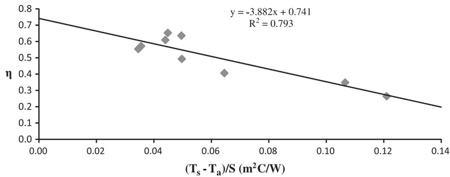
Fig. 9. System efficiency versus loss potential/insolation ratio.
