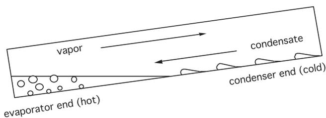
Fig. 3. Schematic of heat pipe operation.
