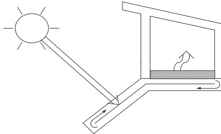
Fig. 1. Isolated gain passive solar system with thermosyphoning collector.
