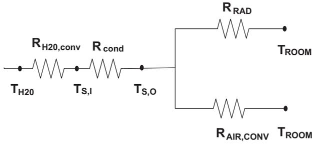
Fig. 5. Thermal resistance network from the thermal mass to the room.
