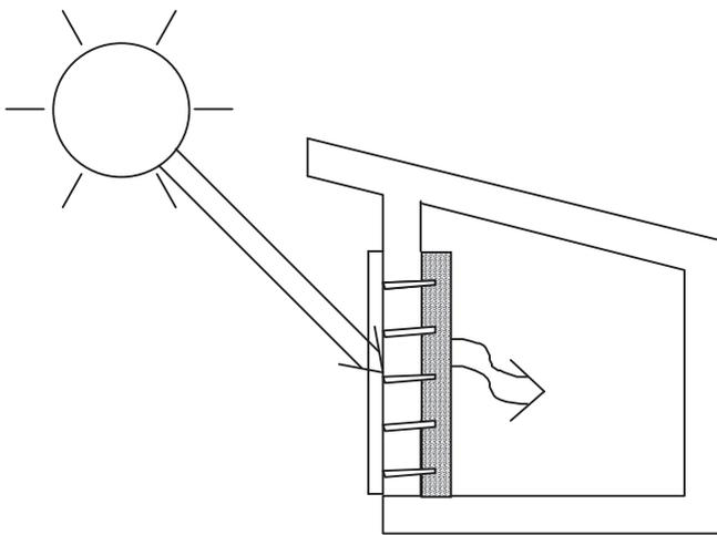
Fig. 2. Isolated gain passive solar heating system with five heat pipes between the absorber and thermal mass.
