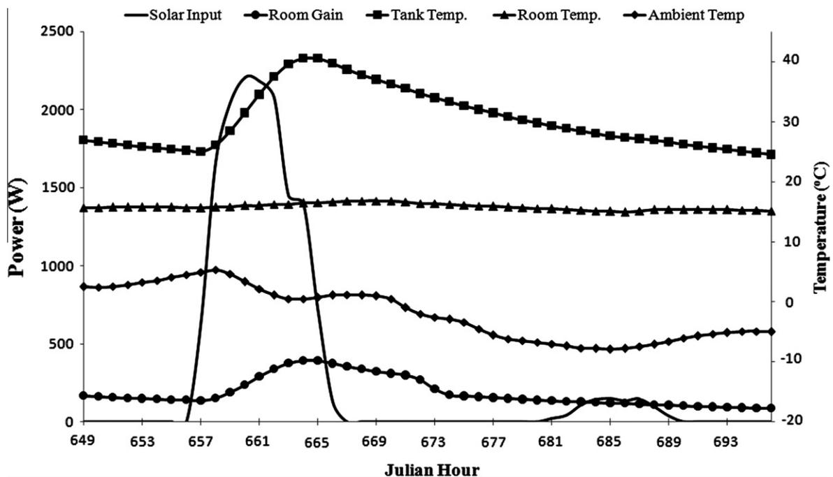
Fig. 6. Average hourly values for insolation, room gain, and tank, room and ambient temperatures for January 28 and 29.
