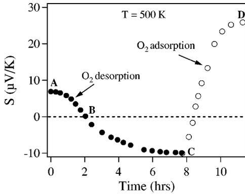
FIG. 2. Thermopower response to vacuum and O<sub>2</sub> (1 atm) at  $T=500$  K. (A→C): Vacuum degassing of a sample initially O<sub>2</sub> doped under ambient conditions for several days. (C→D): Exposure of the degassed sample to 1 atm of O<sub>2</sub> established at C. The TEP remains “locked” at the value  $S=+25\mu\text{V/K}$  at D, i.e., subsequent vacuum degassing has no effect on  $S$ .
