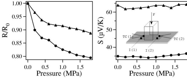
FIG. 1. Uniaxial pressure dependence of the normalized room temperature resistance ( $R/R_0$ ) and thermopower  $S$  for two different SWNT mats. The inset shows the experimental geometry where the applied force  $F$  is perpendicular to the sample.
