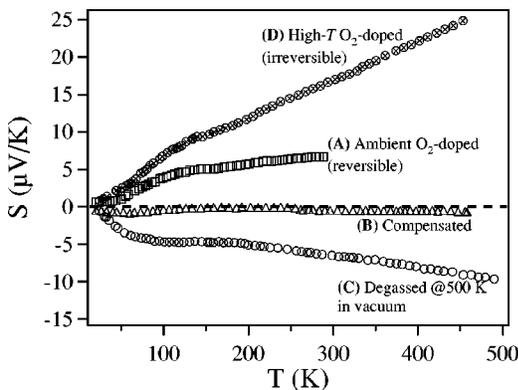
FIG. 3. Temperature dependence of the thermopower  $S$  for a SWNT thin film after successively longer periods of O<sub>2</sub> degassing at  $T=500$  K in vacuum. The labels A, B, and C refer to a vacuum degassing interval indicated in Fig. 2. Curve D is for the same sample exposed to 1 atm O<sub>2</sub> at  $T=500$  K for about 4 hr after being fully degassed to point C.
