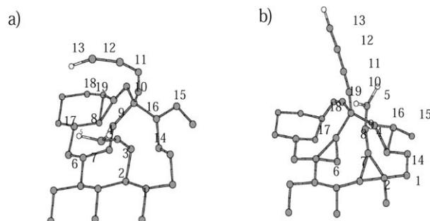
Fig. 5. Representative thin-film fragment from the 50 eV/molecule bombardment simulations termed cluster 3 (a) before and (b) after AM1 geometry optimization.
