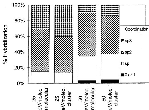
Fig. 7. Summary of the bonding character (hybridization) of the carbon atoms in the hydrocarbon films formed by molecular-beam and cluster-beam deposition.
