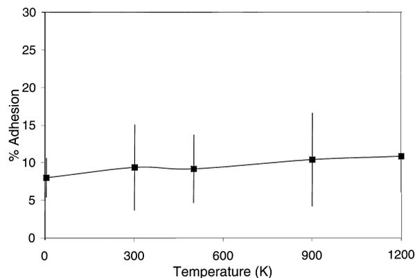
Fig. 2. Percent adhesion of impacting carbon atoms as a function of substrate temperature. The data is averaged over eight trajectories at each temperature.
