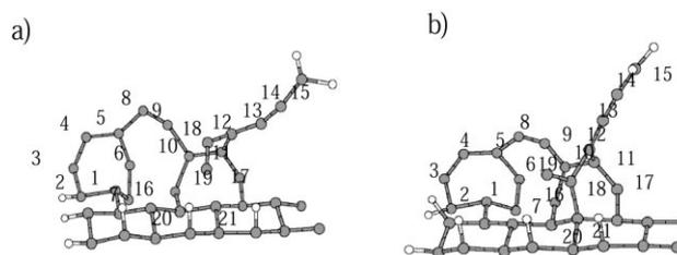
Fig. 6. Representative thin-film fragment from the 50 eV/molecule bombardment simulations termed cluster 4 (a) before and (b) after AM1 geometry optimization.
