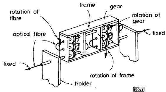
Fig. 2 Endlessly rotatable fractional-wave device (II)
