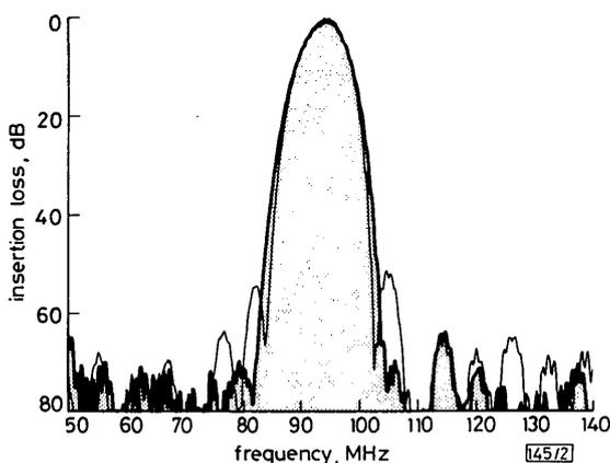
Fig. 2 Filter response before (unshaded) and after (shaded) compensation
