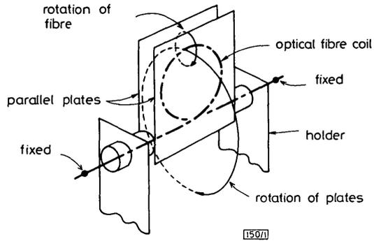
Fig. 1 Endlessly rotatable fractional-wave device (I)
