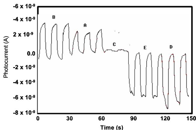
**Figure 3.** The photocurrent of carbon nanotube sheets when the laser spot was on different positions (from A to E) of the sample.
