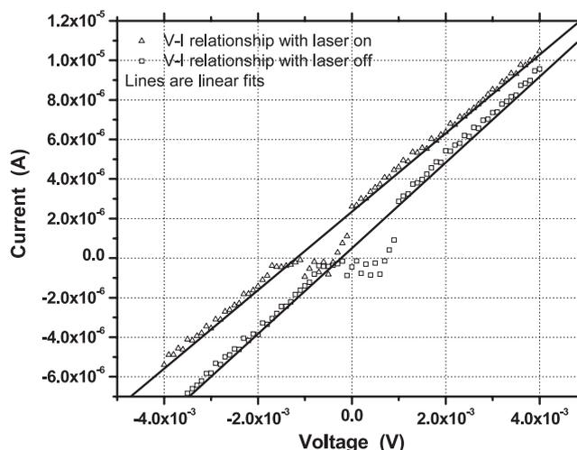
Figure 7.  $V-I$  characteristics with 247 mW laser illumination.
