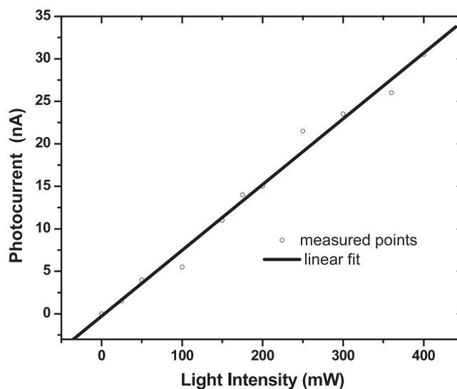
**Figure 4.** The amplitudes of photocurrent as a function of laser intensity. Measurements were done in room atmosphere.
