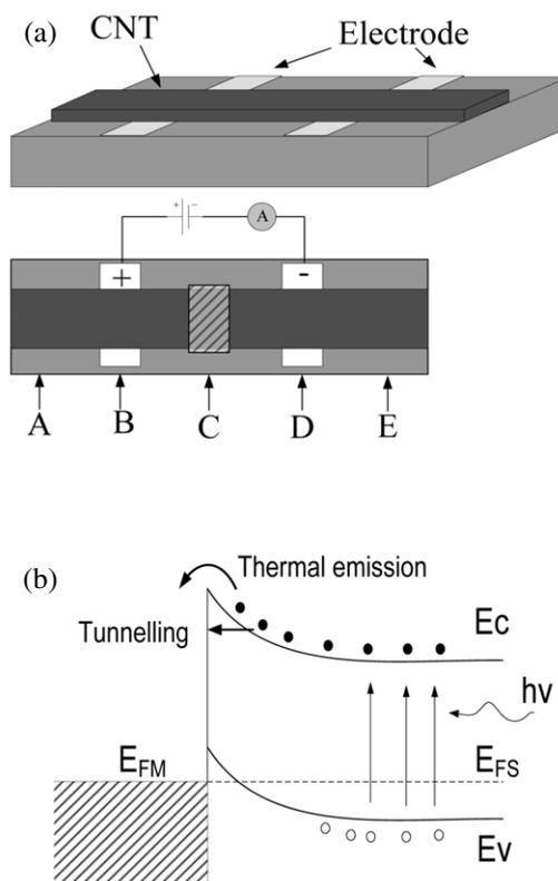
**Figure 2.** (a) Schematic drawing of the carbon nanotube sheets under testing. The bottom part shows the top view of the device. A–E were five testing positions on the sample where a laser spot was pointed. The shaded area indicates that the laser spot was on position C. (b) Band diagram of carbon nanotube (right) in contact with platinum electrodes (left).
