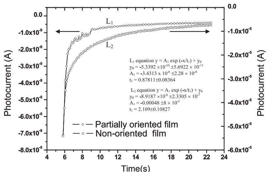
Figure 5. Dynamic responses of photoconductivity and the parameters of their exponential fit. The measurement was done in standard atmosphere pressure, with a light pulse of 25 mHz frequency and 137 mW of laser intensity.
