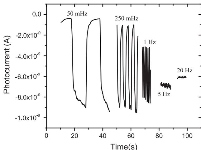
Figure 6. The photocurrent of a nanotube fiber when laser pulses of different frequencies were illuminating the sample. Photocurrent as a function of laser pulse frequencies.
