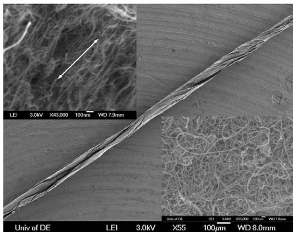
**Figure 1.** SEM image of a partially rolled thin film of carbon nanotubes; inset compares the non-oriented (bottom) and partially oriented (top) samples.
