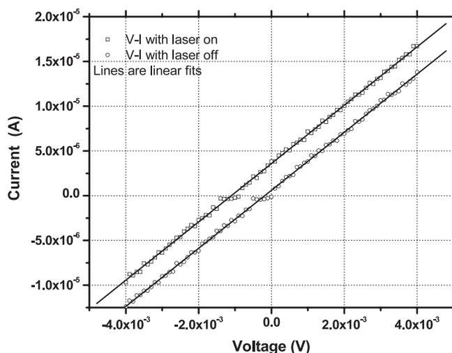
Figure 8.  $V$ – $I$  characteristics with laser on and off in 300 mTorr.
