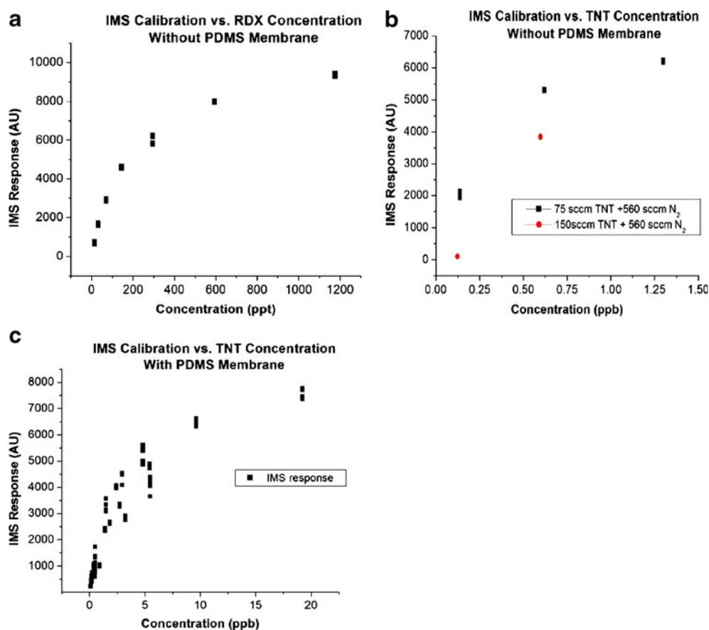
from 40°C to 10°C. Despite the variety of experimental conditions, the variation in the calibration curve is smaller than the case without a membrane and demonstrates the utility of using an inlet membrane to isolate the instrument from environmental effects.
