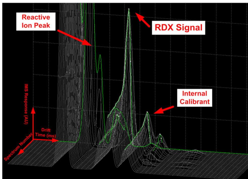
is not as sharp as without an entrance membrane. None the less, the averaged spectrum (plasmagram) indicated a healthy RDX peak at 6.583 ms with a peak height of 2,254. The lack of a calibration curve for RDX with a membrane precludes estimation of the preconcentration factor however a control spectrum with 2.6 PPT taken with the membrane but without the preconcentrators showed that this concentration is below the detection limit of the instrument, i.e. no peak was found.
