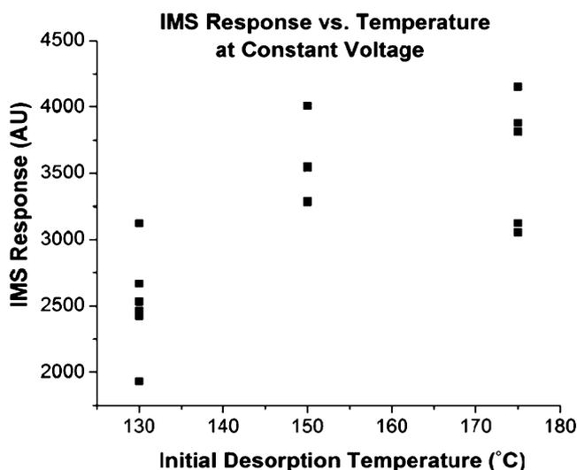
**Fig. 5** Optimization of the desorption temperature with 30 s 142 PPT collection at 190 SCCM. Five data points were taken at each temperature
