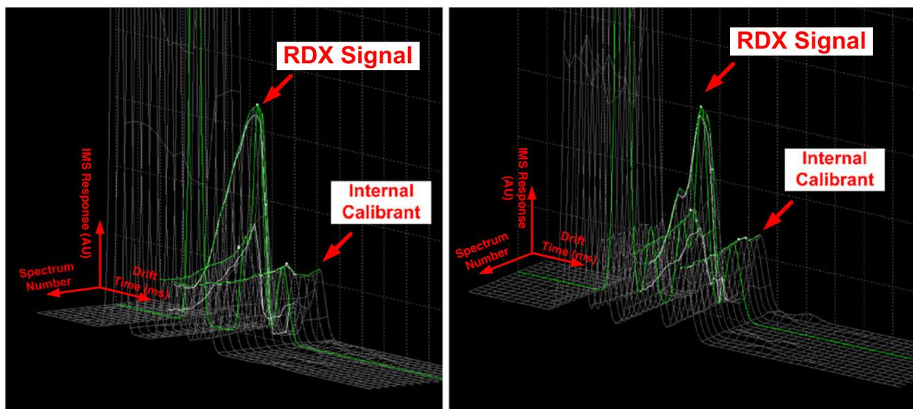
**Fig. 6** Desorption of RDX at constant temperature (*left*) and constant voltage (*right*)
