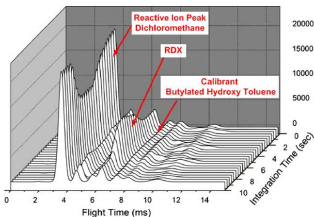
**Fig. 4** Example desorption event for a single preconcentrator. The device was heated for 2 s in constant voltage mode to 150°C after 30 s collection of 14 PPT RDX
