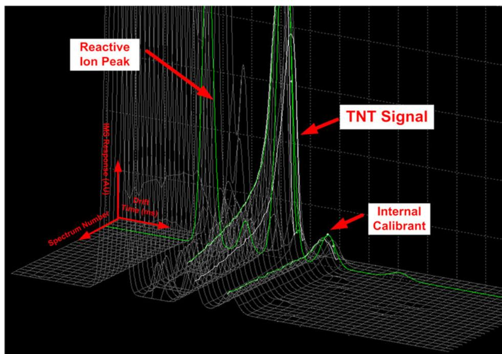
poor calibration for TNT without a membrane it is difficult to accurately measure the preconcentration factor however an estimate of 0.4 PPB would give (400 PPT/13 PPT) a preconcentration factor of 31. The devices were left on after desorption and 45 s later a second spectrum showed a TNT peak height of 186, well below the default alarm level of 250.
