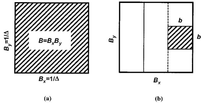
**Fig. 2** Available spatial bandwidth of SLMs and usable spatial bandwidth (shaded regions) of various encoding algorithms with the plots in the Fourier transform or reconstruction plane of the SLM: (a) available spatial bandwidth  $B$  of an  $n \times n$  pixel array of pitch  $\Delta$  in both  $x$  and  $y$  and (b) usable bandwidth  $B/9$  for Burckhardt's method under the constraint that the usable area is of square aspect.<sup>1</sup>
