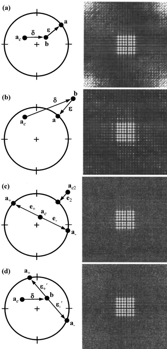
**Fig. 9** Encoding method and corresponding simulated far-field intensity patterns for (a) ED,  $\gamma=1$ ; (b) ED,  $\gamma=1.5$ ; (c) MD-PRE,  $\gamma=1.4$ ; and (d) ED-PRE,  $\gamma=1.3$ ,  $\chi=0.6$ . Images are saturated so that the maximum grayscale value (full white) is 3% of the average intensity of the 49 spots.<sup>20</sup>
