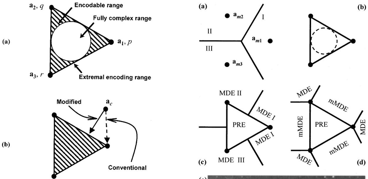
**Fig. 6** Ternary pseudorandom encoding showing (a) PRE encoding and fully complex range,<sup>4</sup> and (b) distinction between MD-PRE (conventional) and mMD-PRE (modified) for a ternary SLM (Ref. 17).
