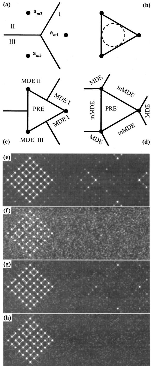
**Fig. 7** Encoding methods (a) MDE, (b) PRE, (c) MD-PRE, and (d) mMD-PRE and respective simulated far-field intensity patterns for (e) MDE with  $\gamma=\infty$ , (f) PRE with  $\gamma=0.5$ , (g) MD-PRE with  $\gamma=0.80$ , and (h) mMD-PRE with  $\gamma=0.95$ . To bring out the background noise the maximum grayscale value (full white) is 30% of the average intensity of the 49 spots. Approximately  $40 \times 107$  resolution cells of the full  $128 \times 128$  NRB are shown.<sup>17</sup>
