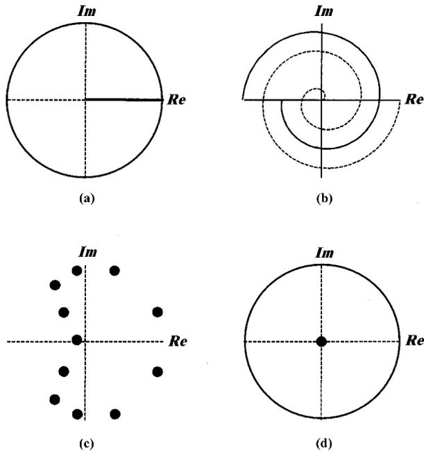
**Fig. 1** Various possible modulation ranges for SLMs: (a) phase-only and amplitude-only (thick line); (b) coupled amplitude phase, which have continuous phase ranges of  $2\pi$  (solid line) and  $4\pi$  (dashed line); (c) quantized; (d) bi-amplitude phase specifically showing amplitudes of unity and zero.<sup>1</sup>
