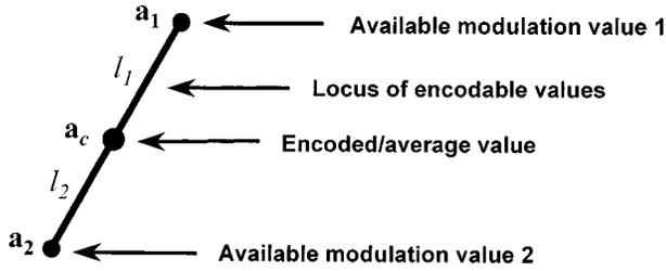
**Fig. 5** Geometry of pseudorandom biamplitude encoding. Any desired value  $\mathbf{a}_c$  between the two available modulation values  $\mathbf{a}_1$  and  $\mathbf{a}_2$  can be encoded by pseudorandom encoding.<sup>4</sup>
