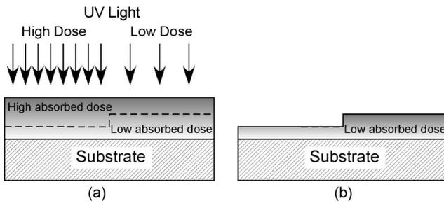
Fig. 1. (a) Schematic of a positive photoresist exposed to a high dose and a low dose for grayscale lithography. (b) Resulting photoresist profile after development.
