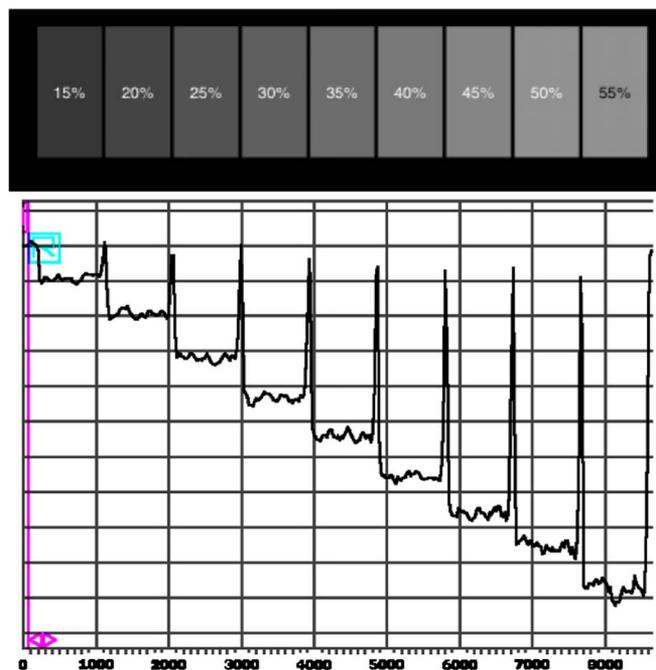
Fig. 5. (Top) Bitmap file used to characterize the grayscale lithography process. (Bottom) Contact profilometer line scan of the developed HD-8820 film, after exposure to the bitmap file shown above, but before the final cure. The peaks in the profilometer scan are due to (black lines in the bitmap file) the unexposed regions separating the regions with different grayscale levels.
