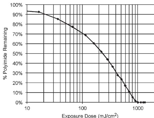
Fig. 4. This graph shows the percentage of polyimide that remained after the development step as a function of the total exposure dose.
