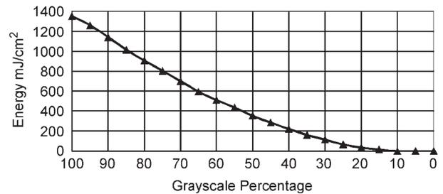
Fig. 3. Measured light output from the SF-100 as a function of the input grayscale percentage, integrated over a 10-s exposure. Both the *i*-line (365 nm) and *h*-line (405 nm) were measured. White corresponds to 100%, and black corresponds to 0%.
