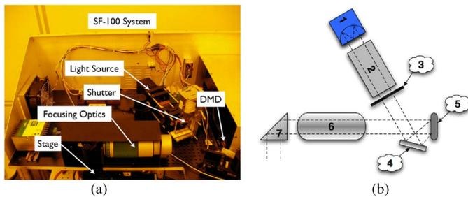
Fig. 2. (a) Layout of SF-100 DMD-based maskless lithography system used for grayscale exposures. (b) Schematic of the DMD-based maskless lithography system. Light from (1) the mercury lamp passes through (2) collimating optics and (3) a shutter. After reflecting off (4) a mirror, the light is reflected off (5) the smart filter, which contains the DMD array. Finally, the light goes through (6) the imaging optics and is reflected off (7) a mirror to the substrate on the stage below the optics.
