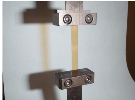
Fig. 8. Photograph of strip of polyimide undergoing tensile testing.
