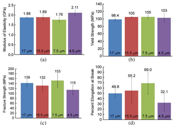
Fig. 9. Comparison of the averages of (a) the modulus of elasticity, (b) the yield strength, (c) the fracture strength, and (d) the percent elongation at break for polyimide samples of thicknesses  $17$ ,  $15.5$ ,  $7.5$ , and  $4.5\ \mu\text{m}$ .
