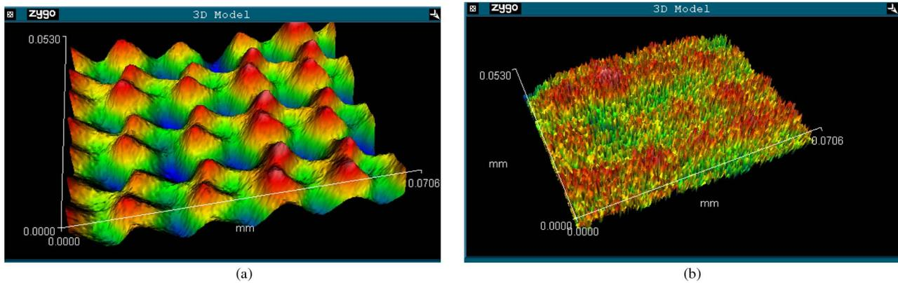
Fig. 7. Three-dimensional profile of surface roughness of the polyimide, measured with a Zygo white light interferometer. (a) Prior to the final cure, peaks with a spacing of  $15\ \mu\text{m}$  are observed, corresponding to the individual micromirrors in the DMD array. The surface roughness  $R_a$  is  $11.2\ \text{nm}$ . (b) After the final cure, the large peaks that were present before the cure have nearly been eliminated. The surface roughness  $R_a$  is reduced to  $4.4\ \text{nm}$ .
