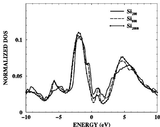
FIG. 2. A comparison of the normalized electronic density of states of relaxed  $\text{Si}_{200}$ ,  $\text{Si}_{800}$  and  $\text{Si}_{2000}$ , respectively. No discernible gap is seen in this case, where the energy of HOMO level is fixed at zero.
