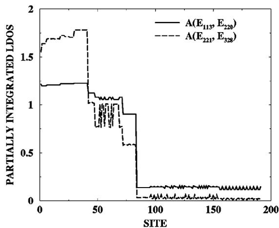
FIG. 6. Partially integrated local density of states is plotted at the sites of unrelaxed  $\text{Si}_{83}\text{H}_{108}$  cluster.
