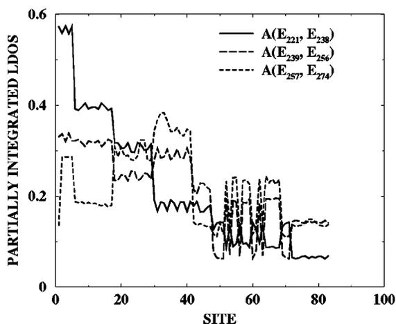
FIG. 5. Partially integrated local density of states is plotted at the sites of the unrelaxed  $\text{Si}_{83}$  cluster for energy eigenvalue index 221–274 in steps of 18.
