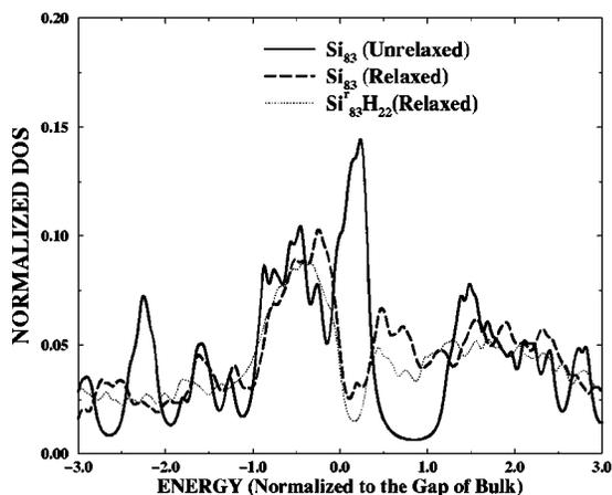
FIG. 9. A comparison of the normalized electronic density of states of unrelaxed  $\text{Si}_{83}$ , relaxed  $\text{Si}_{83}$ , and relaxed  $\text{Si}_{83}\text{H}_{22}$  whose remnant dangling bonds are saturated with hydrogen atoms, respectively.
