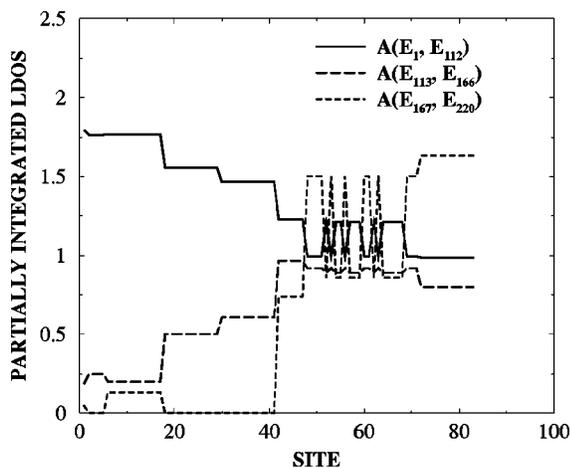
FIG. 4. Partially integrated local density of states is plotted for three different energy intervals (two below and one above the HOMO level) at the sites of the unrelaxed  $\text{Si}_{83}$  cluster.
