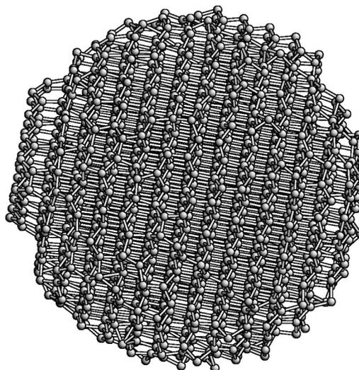
FIG. 1. Optimized structure of Si<sub>2000</sub> as obtained by the O(N)/NOTB-MD method.
