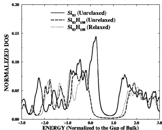
FIG. 3. A comparison of the normalized electronic density of states of the unrelaxed  $\text{Si}_{83}$  unrelaxed  $\text{Si}_{83}\text{H}_{108}$ , and relaxed  $\text{Si}_{83}\text{H}_{108}$ , respectively. The energy of HOMO for each case is set at zero.
