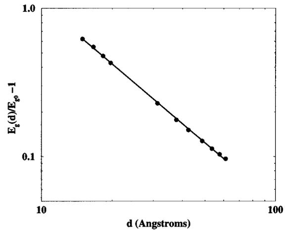
FIG. 11. The energy gap of the hydrogen-passivated silicon cluster as a function of the size of the cluster.
