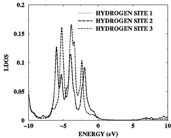
FIG. 8. Local density of states at hydrogen sites which typically saturate three dangling bonds associated with an exterior Si atom.
