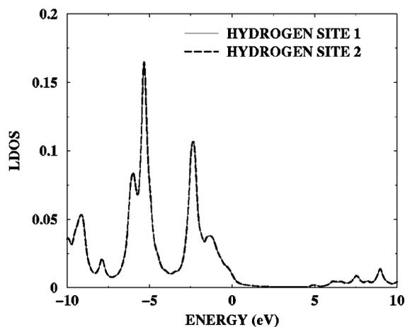
FIG. 7. Local density of states at hydrogen sites which typically saturate two dangling bonds associated with an exterior Si atom.
