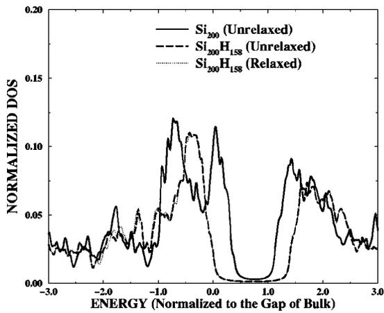
FIG. 10. A comparison of the normalized electronic density of states of unrelaxed  $\text{Si}_{200}$ , unrelaxed  $\text{Si}_{200}\text{H}_{158}$ , and relaxed  $\text{Si}_{200}\text{H}_{158}$ .
