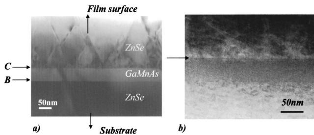
FIG. 1. (a) Bright-field TEM image shows ZnSe/Ga<sub>1-x</sub>Mn<sub>x</sub>As/ZnSe multilayers. Interface A is ZnSe/GaAs-substrate (not shown here), B and C are the interfaces of ZnSe/Ga<sub>1-x</sub>Mn<sub>x</sub>As/ZnSe, as marked in the figure. Stacking faults are observed at interface C. (b) Annular dark-field STEM image of the interfaces that shows a dark line at interface C, as marked by the arrow.
