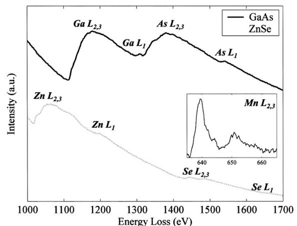
FIG. 3. Typical EEL spectra taken from Ga<sub>1-x</sub>Mn<sub>x</sub>As and ZnSe layers. Inset is Mn L<sub>2,3</sub> edge obtained from the Ga<sub>1-x</sub>Mn<sub>x</sub>As layer.
