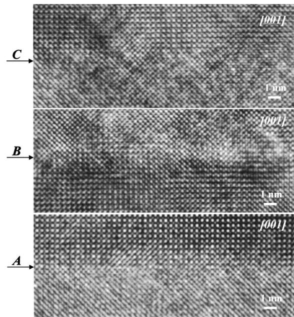
FIG. 2. HRTEM images showing interfaces (A) ZnSe/GaAs-substrate, (B) Ga<sub>1-x</sub>Mn<sub>x</sub>As on ZnSe, and (C) ZnSe on Ga<sub>1-x</sub>Mn<sub>x</sub>As.
