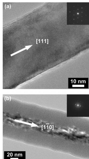
FIG. 2. HRTEM images of (a) TMB-doped ( $[B:Si]_{\text{gas}} = 1.6 \times 10^{-2}$ ) SiNW with [111] growth orientation. A thin oxide layer was observed on the outer surface. (b)  $B_2H_6$ -doped ( $[B:Si]_{\text{gas}} = 1.4 \times 10^{-2}$ ) SiNW consisting of a crystalline Si core surrounded by an amorphous Si shell.
