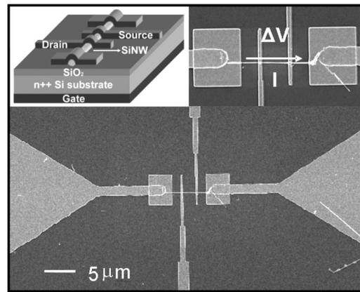
FIG. 3. FESEM image of the back-gated test structure used for four-point resistance and gate-dependent conductance measurements. A 3D schematic of the back-gated test structure is shown as an inset at the top left along with a high magnification image of the SiNW at the top right.
