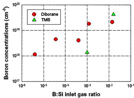
FIG. 1. (Color online) Boron concentration in SiNWs obtained by SIMS measurements as a function of the B:Si ratio in the inlet gas.
