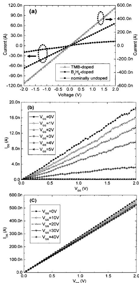
FIG. 4. (a) Two-point  $I$ - $V$  of nominally undoped,  $B_2H_6$ -doped (left current axis), and TMB-doped SiNWs (right current axis). Gate-dependent  $I$ - $V$  of the same (b) nominally undoped and (c) TMB-doped SiNW. The topmost curve in (b) and (c) plots are measured under  $V_{GS}=0$  V. The gate voltage step for the nominally undoped SiNWs is  $V_{GS}=+1$  V and that of the TMB-doped SiNWs is  $V_{GS}=+10$  V.
