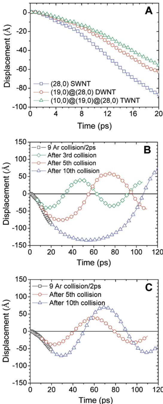
**Figure 3.** (A) Comparison of the displacements of a SWNT, DWNT, and TWNT after the same number of collision events (up to 10) with Ar. (B) The displacement of a (28,0) SWNT, and (C) the displacement of a (10,0)@(19,0)@(28,0) TWNT after collision events with Ar and relaxation.
