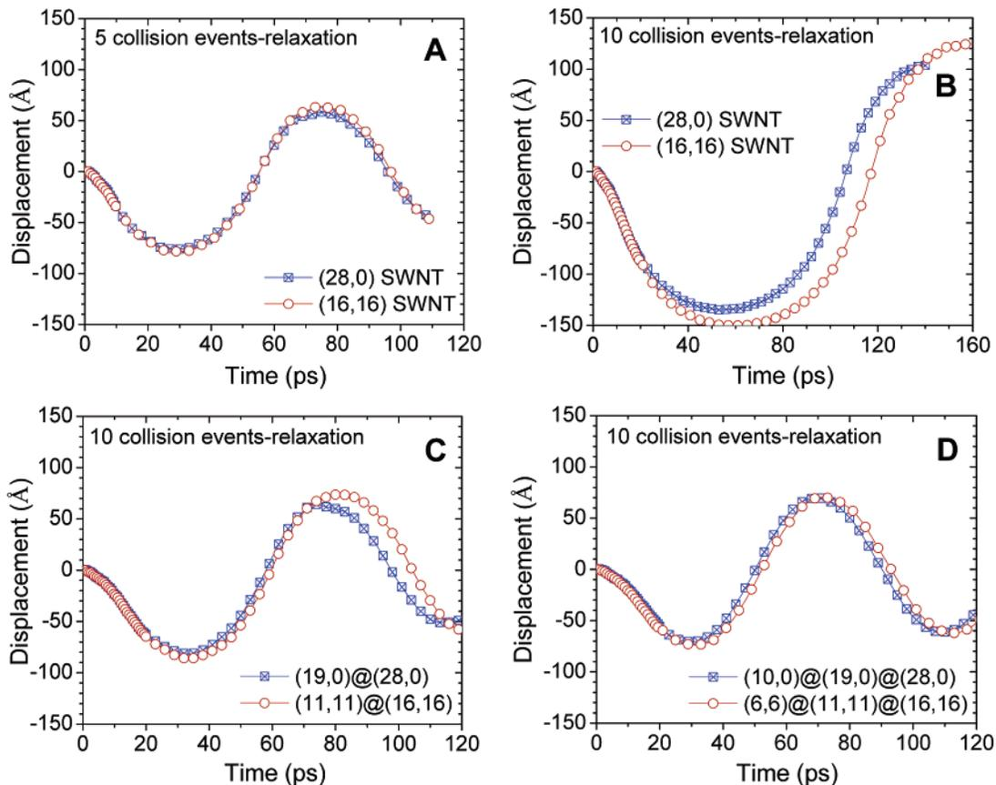
**Figure 4.** Relative displacements of armchair and zigzag nanotubes after multiple collision events with Ar. (A) Five collision events followed by relaxation and (B) ten collision events followed by relaxation of (28,0) and (16,16) SWNTs. (C) Ten collision events followed by relaxation of (19,0)@(28,0), and (10,10)@(16,16) DWNTs. (D) Ten collision events followed by relaxation of (10,0)@(19,0)@(28,0), and C) (10,0)@(11,11)@(16,16) TWNTs.
