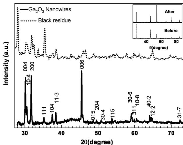
Fig. 1. XRD pattern of the samples collected from different parts of the reactor; white color web-like structures at the edges of the boat (solid line) and black deposit on the inner walls of the reactor wall in the cold part in the down stream (dotted line). Also shown in the inset is the XRD pattern of the lump of black residue in the center of the boat. XRD pattern of the GaAs powder is also shown in the inset for comparison.
