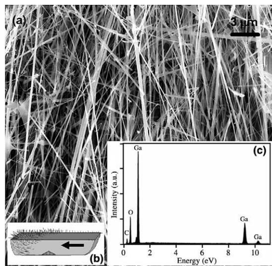
Fig. 2. (a) SEM image of the material obtained from the inner walls of the quartz boat synthesized using Te doped GaAs powder. (b) Shown in the inset is the schematic diagram of the quartz boat with resulting products after the growth. (c) EDX spectrum shows peaks corresponding to Ga, O and C.
