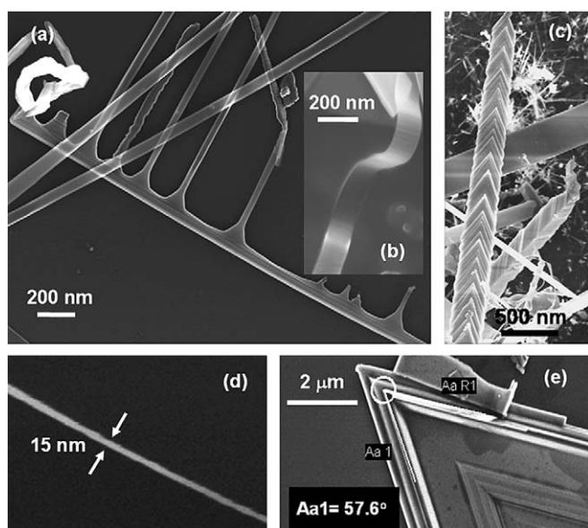
Fig. 3. SEM images of various  $\text{Ga}_2\text{O}_3$  nanowire morphologies: (i) resulted from Te assisted growth; (a) comb-like structure, (b) nanoribbon, (c) herringbone structure, (d) small diameter ( $\sim 15$  nm) nanowire resulted from S assisted growth and (e) larger size of herringbone structure.
