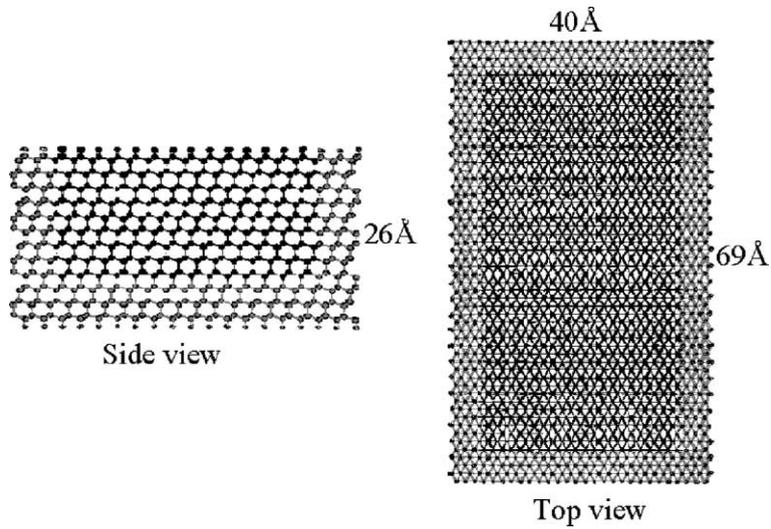
Fig. 1. The arrangement of thermostat atoms (grey) and normal atoms (black) within the substrate.
