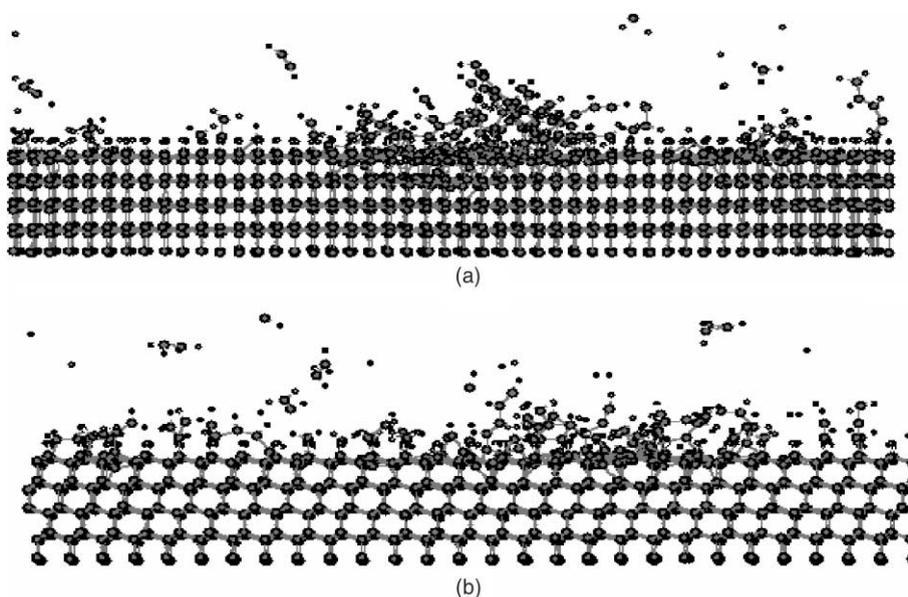
Fig. 4. Snapshots from the MD simulations of the nucleated thin films as a result of ethylene cluster beam deposition: (a) from a simulation where the total incident energy is 50 eV/cluster-molecule along the (I) crystallographic orientation at  $15^\circ$  and (b) from a simulation where the total incident energy is 50 eV/cluster-molecule along the (II) crystallographic orientation at  $45^\circ$ .
