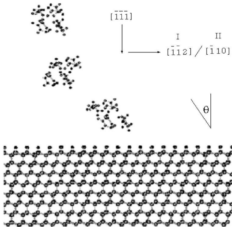
Fig. 2. A representative snapshot of the system prior to deposition of the cluster beam (only part of the cluster beam and the substrate are shown for clarity).
