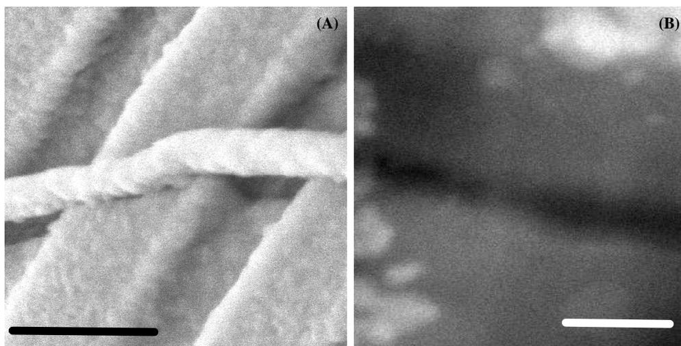
**Figure 2.** (A) SEM image of an MWCNT suspended on a patterned substrate after Al deposition, showing a shadow underneath the MWCNT. The scale bar is 300 nm. (B) 6 nm shadow projected under a  $\sim 20$  nm diameter MWCNT, as seen by STEM. The scale bar is 20 nm.
