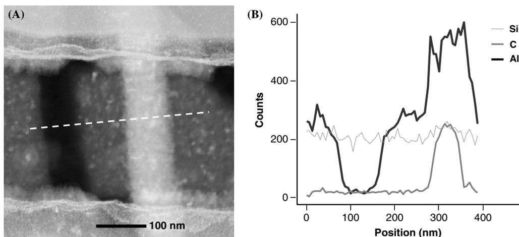
**Figure 3.** Representative (A) STEM image and (B) EDS line scan (dashed line in (A)) for suspended CNT shadow lithography. The TEM substrate is tilted by  $15^\circ$  relative to the electron beam axis so as to image both the MWCNT and its shadow gap. The evaporation shutter distance was 7 cm; the e-beam resist thickness was 400 nm.
