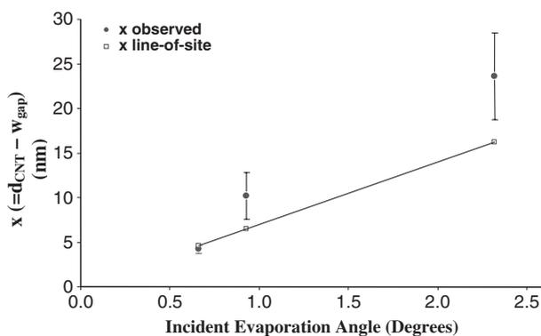
**Figure 4.** CNT diameter ( $d_{\text{CNT}}$ ) minus shadow width ( $w_{\text{gap}}$ ) versus incident evaporation angle.
