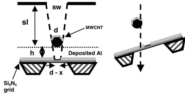
**Figure 1.** Incident angle dependence of shadow formation under suspended MWCNT. STEM can image both the MWCNT and shadow by tilting the sample. The left-hand diagram shows the deposition geometry, and the right-hand diagram shows the scheme for electron beam imaging. See the text for an explanation of the dimensional parameters.
