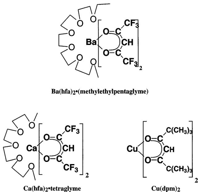
FIG. 5. Precursor molecules utilized in the MOCVD deposition of BaCaCuO(F) thin films. Ba(hfa)<sub>2</sub>·mep (hfa = hexafluoroacetylacetonate, mep = methylethylpentaglyme), Ca(hfa)<sub>2</sub>·tet (tet = tetraglyme), and Cu(dpm)<sub>2</sub> (dpm = dipivaloylmethanate). The Ba and Ca precursors are liquid under typical film deposition conditions.
