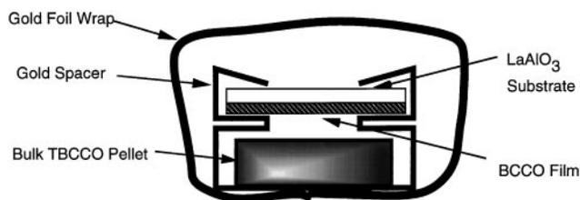
FIG. 4. Diagram of the annealing scheme used to form films of the Tl-2212 superconductor. The large bulk pellet acts as a source for a near-equilibrium vapor pressure of  $Tl_2O$ .
