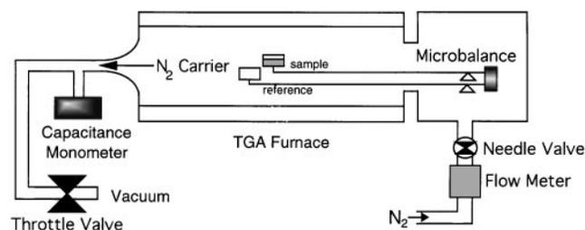
FIG. 1. Schematic diagram of the horizontal, reduced pressure thermogravimetric analysis (TGA) instrumentation utilized in the study of MOCVD precursor volatility.
