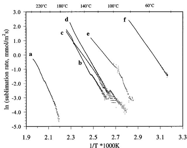
FIG. 8. Comparison of volatilities of several common MOCVD precursors in reduced pressure TGA experiments. Evaporation rates are adjusted to a diffusion distance of 1.7 mm in 5 Torr total pressure  $N_2$ . (a)  $Ba(dpm)_2$ , (b)  $Ba(hfa)_2 \cdot tet$ , (c)  $Ba(hfa)_2 \cdot mep$ , (d)  $Cu(dpm)_2$ , (e)  $Ca(hfa)_2 \cdot tet$ , and (f)  $Cu(hfa)_2$ .
