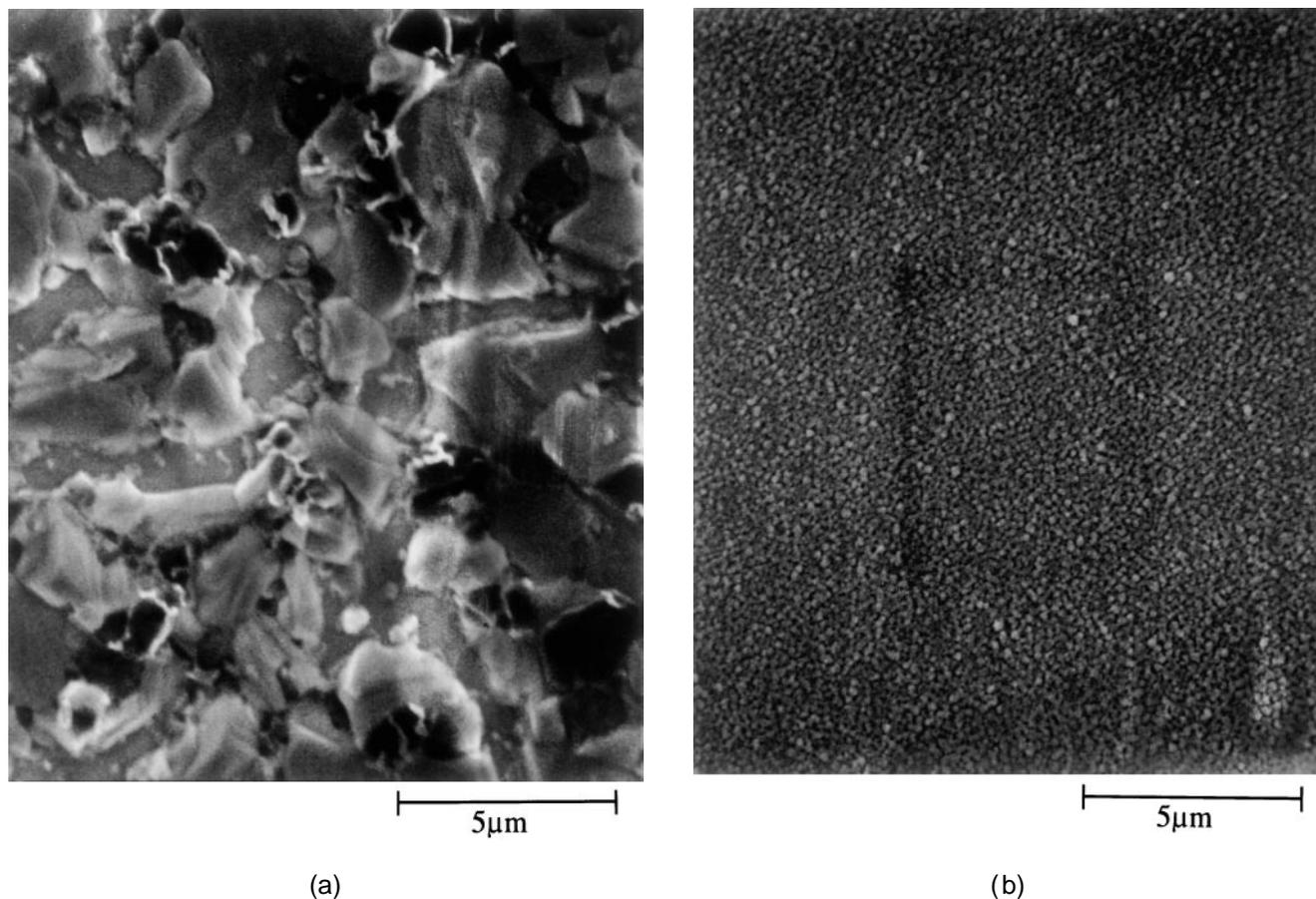
FIG. 15. (a) SEM image of a fluorine-free, MOCVD-derived BaCaCuO film deposited at a substrate temperature of 780 °C showing rough surface morphology. (b) SEM image of the surface morphology of a BCCO(F) film grown on (110) LaAlO<sub>3</sub> under typical MOCVD deposition conditions with a 500 °C substrate temperature.
