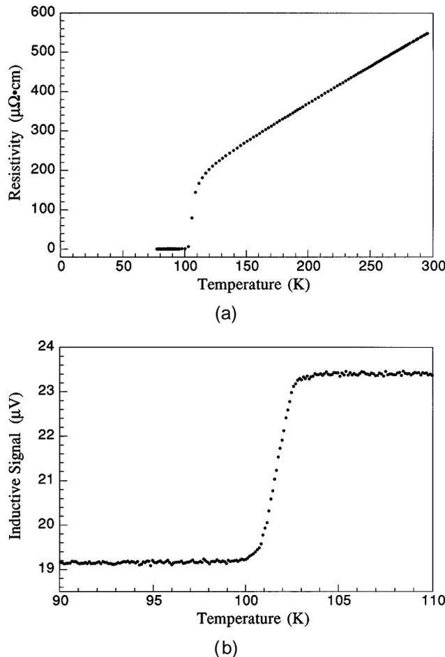
FIG. 19. (a) Variable-temperature, four-probe resistivity data for a MOCVD-derived Tl-2212 film showing  $T_c = 103$  K. (b) An inductive  $T_c$  measurement on a Tl-2212 film showing a sharp critical transition through the sample.
