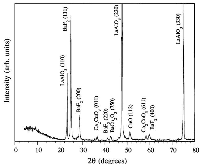
FIG. 13.  $\theta$ - $2\theta$  x-ray diffraction scan of a BaCaCuO(F) film grown on (110)  $\text{LaAlO}_3$  under conditions given in Table I.
