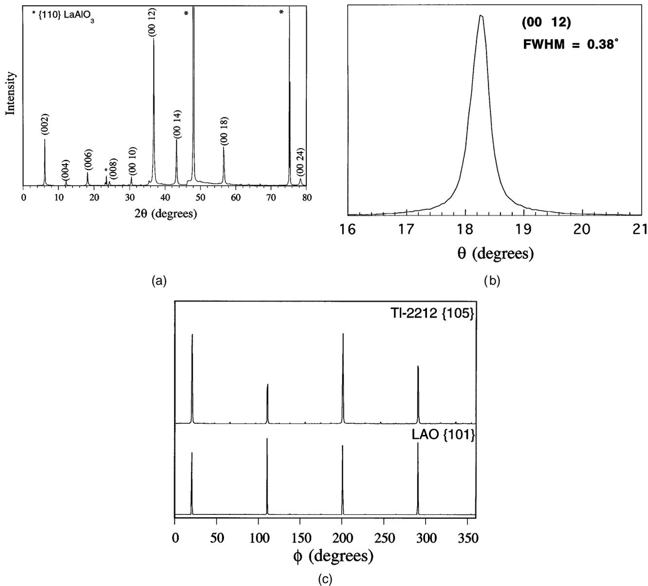
FIG. 17. (a)  $\theta$ - $2\theta$  x-ray diffraction pattern of a MOCVD-derived Tl-2212 thin film grown on (110) LaAlO<sub>3</sub>. (b)  $\theta$ -rocking curve of the (0012) reflection of a MOCVD-derived Tl-2212 thin film grown on (110) LaAlO<sub>3</sub> [pseudo cubic (100)]. (c) In-plane  $\phi$ -scan of the {105} reflections of a MOCVD-derived Tl-2212 showing alignment with the underlying pseudo-cubic {101} reflections of the LaAlO<sub>3</sub> substrate and indicating epitaxial growth.
