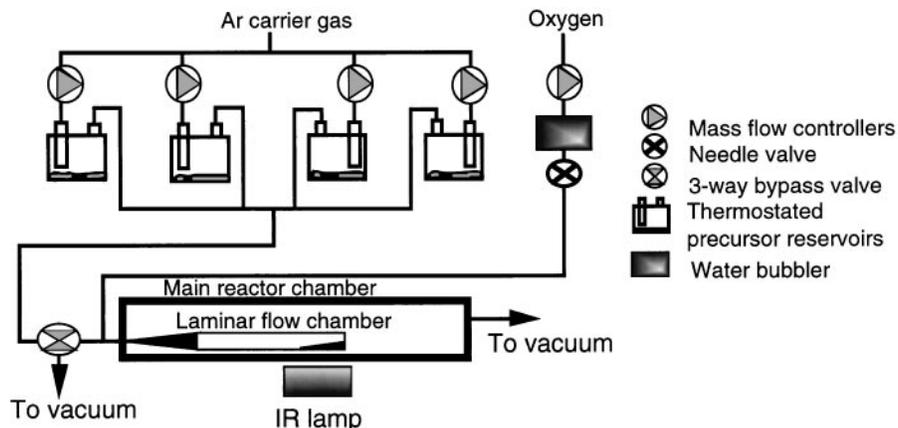
FIG. 2. Schematic diagram of the horizontal hot-wall MOCVD film growth reactor utilized in this study.
