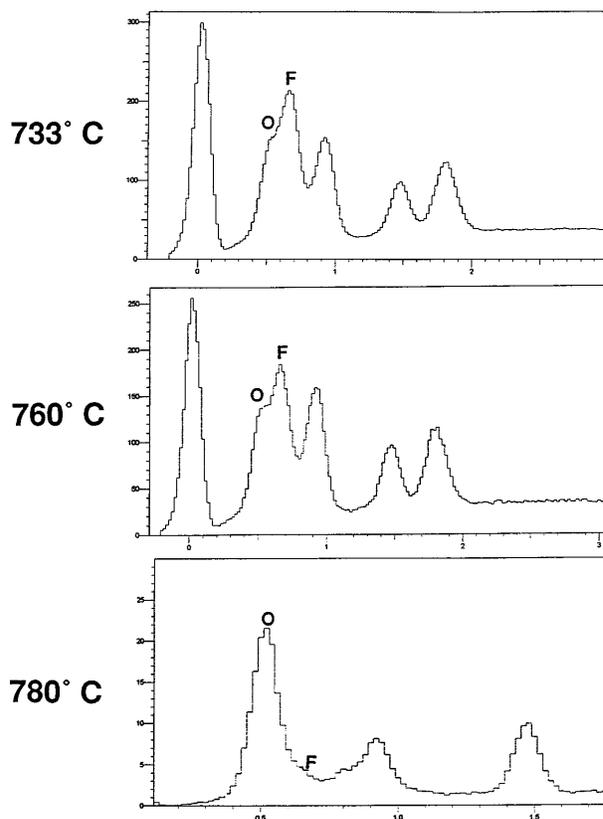
FIG. 14. Windowless EDX spectra showing BaCaCuO(F) film fluoride content at the film growth temperatures indicated. Growth conditions: 150 sccm Ar carrier, 100 sccm  $\text{O}_2$ , 250 sccm  $\text{H}_2\text{O}$ , and 5 Torr total pressure.
