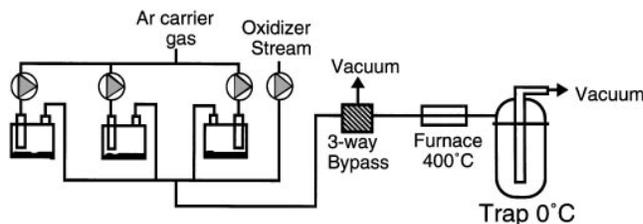
FIG. 3. Schematic of the apparatus employed to trap metal-organic by-products produced from  $Ba(hfa)_2 \cdot mep$ ,  $Ca(hfa)_2 \cdot tet$ , and  $Cu(dpm)_2$  in MOCVD growth experiments.
