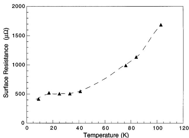
FIG. 21. Temperature dependence of the microwave surface resistance ( $R_s$ ) of a pair of MOCVD-derived TI-2212 thin films at 10 GHz as measured by a parallel plate resonator technique.
