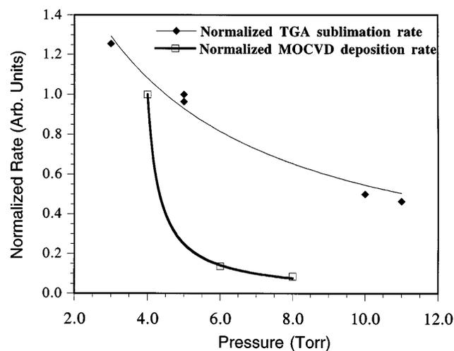
FIG. 11. Deposition rate of BaF<sub>2</sub> films versus system pressure showing the large effect of carrier velocity on film deposition rate. Pressure is regulated by throttle valve on the reactor exhaust. Conditions: 500 sccm total flow and 500 °C substrate temperature. For comparison, normalized TGA evaporation rate data for of Ba(hfa)<sub>2</sub>•mep at 120 °C as a function of pressure are shown.
