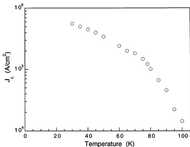
FIG. 20. Transport-measured critical current density as a function of temperature for a MOCVD-derived TI-2212 thin film. Measurements were performed on a 80  $\mu\text{m}$  wide bridge using a 10  $\mu\text{V}/\text{cm}$  criterion.
