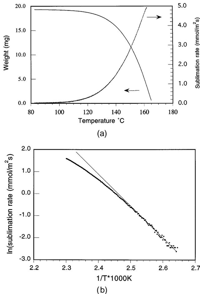
FIG. 6. (a) Typical weight loss and derivative (mass with respect to time) data for the reduced pressure TGA of the MOCVD precursor Cu(dpm)<sub>2</sub> at 5 Torr total pressure, N<sub>2</sub> carrier. (b) Arrhenius plot of the sublimation rate versus temperature showing deviation from linearity principally due to diffusion effects (the straight line is drawn as a guide to the eye).
