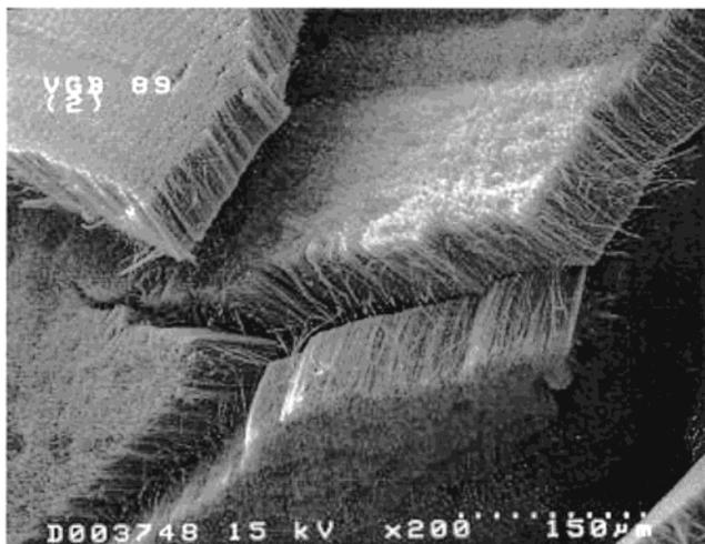
**Figure 1.** SEM picture showing MWNT length.
