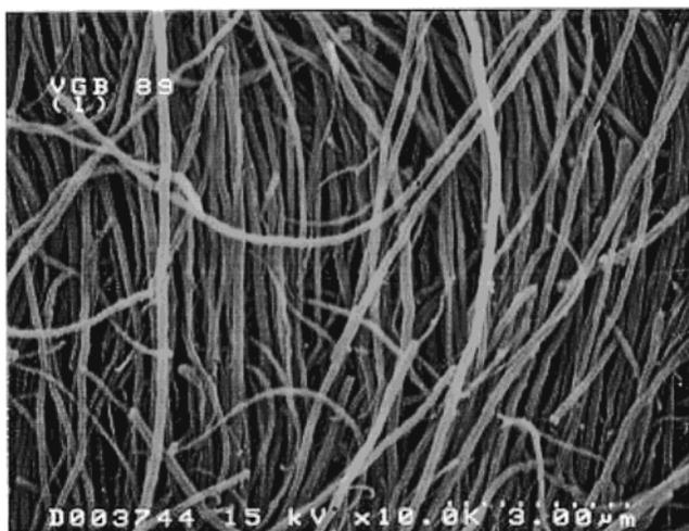
**Figure 2.** SEM picture showing the variety of outer diameter for MWNTs.
