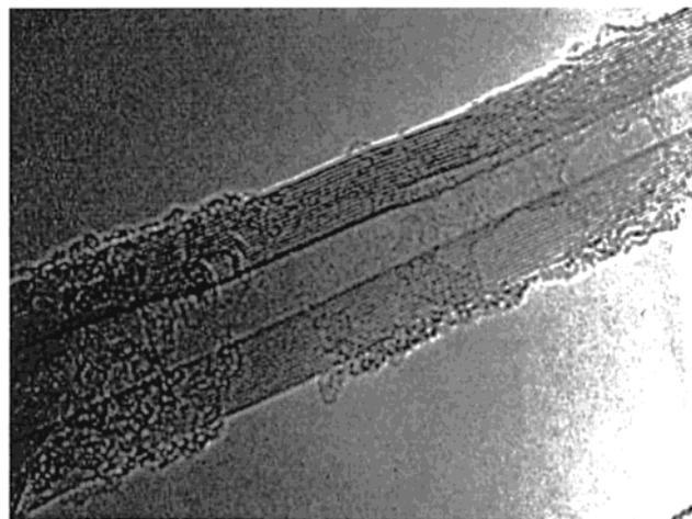
**Figure 3.** TEM picture showing the pore at the core of a MWNT.
