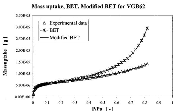
**Figure 8.** Comparison of BET and modified BET equations with VGB62 sorption data.**Table 3. Comparison of  $n_m$  (Monolayer Coverage) Estimated by Using Three Different Methods**
