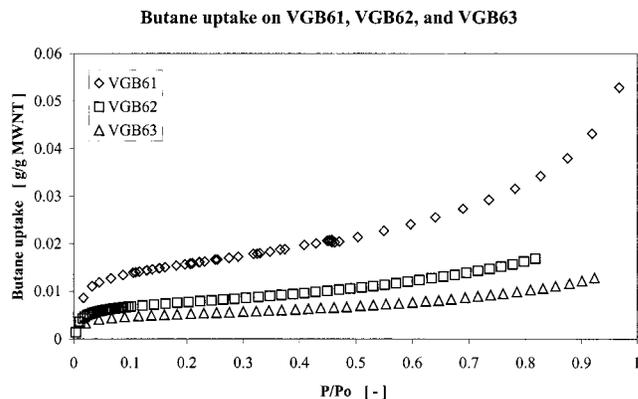
**Figure 7.** Butane sorption isotherms for three MWNT samples.
