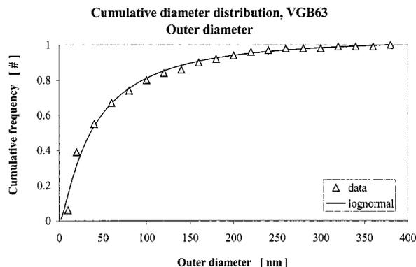
**Figure 6.** Graph showing a log-normal fit to cumulative diameter distribution for VGB63, external diameter.
