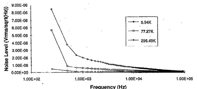
FIG. 3. Input referred noise voltage vs frequency at 300, 77, and 4.2 K.
