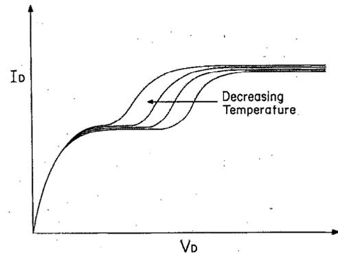
FIG. 2. The current kink in the MOSFET *I*-*V* curve at low temperatures is schematically shown here. Note that the critical voltage decreases with decreasing temperature. (Adapted from Ref. 21.)
