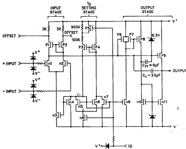
FIG. 1. Functional diagram for the ICL7611-DMTV opamp. *N*-channel MOSFETs are designated as *nX* and *p*-channel as *PX*.
