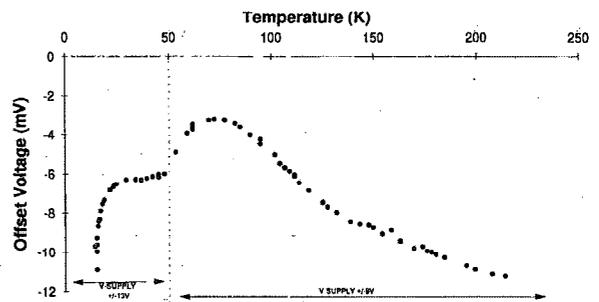
FIG. 8. Input offset voltage plotted against temperature with the offset nulling capability disconnected. The specification for normal temperatures is 20 mV.
