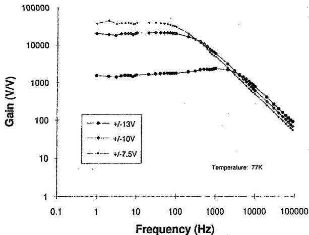
FIG. 7. Open-loop gain of a typical opamp at 77 K at supply voltages of  $\pm 7.5$ ,  $\pm 10$ , and  $\pm 13$  V.
