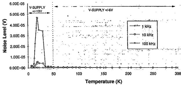
FIG. 4. Input referred noise voltage vs temperature at 1, 10, and 100 kHz. Note the drastic increase in noise between 10 and 40 K.
