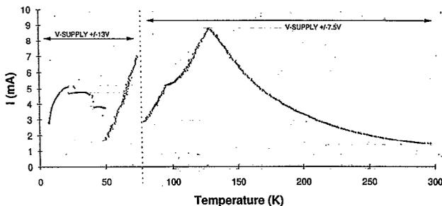
FIG. 5. Quiescent current of a typical opamp as measured at the positive supply with respect to temperature.
