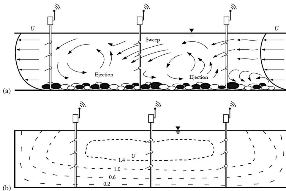
**Fig. 8.** (a) Depiction of VBS measuring macroturbulence in a stream; (b) VBS measuring time-averaged flow to construct  $U$  isovels in  $\text{cm s}^{-1}$  for a cross section
