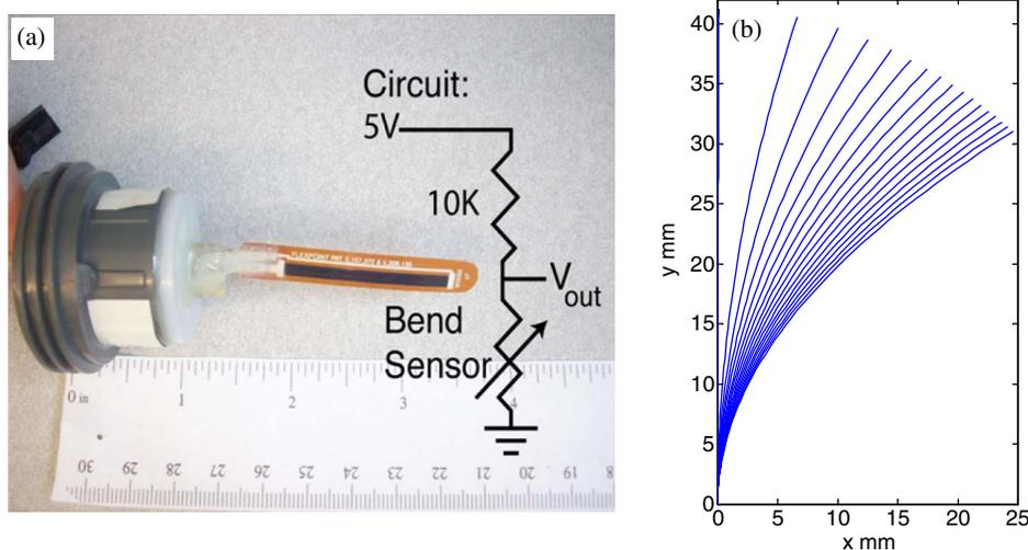
**Fig. 1.** (a) Photograph of a VBS with a depiction of electronic behavior; (b) approximate deflected shape of the VBS in bending when increasing from 0 to 80 cm s<sup>-1</sup> in 5 cm s<sup>-1</sup> increments
