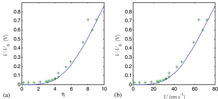
**Fig. 5.** (a) VBS voltage plotted against nondimensional velocity  $\eta$ ; (b) VBS voltage plotted against time-averaged approach velocity
