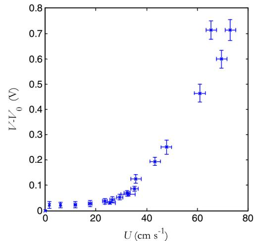
Fig. 3. Time-averaged approach velocity versus output voltage
