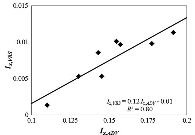
Fig. 7. Turbulent intensity comparison for VBS voltage and ADV streamwise velocity
