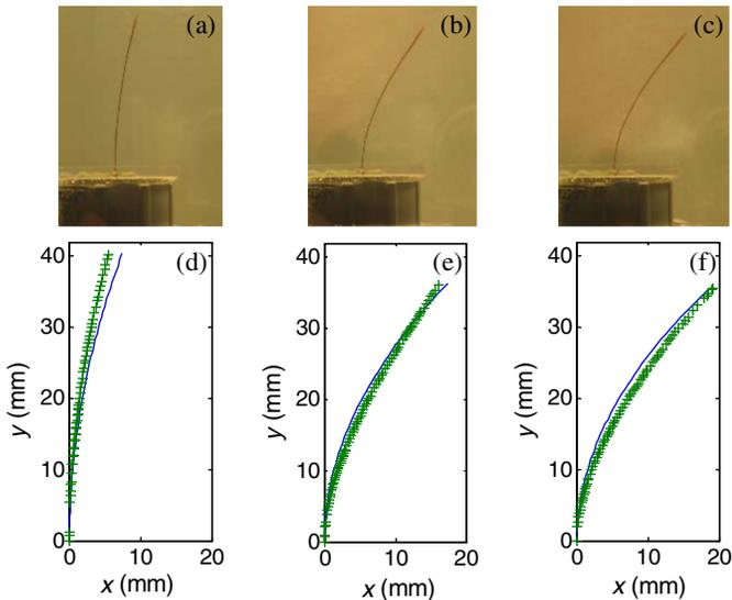
**Fig. 4.** Photographs of the VBS in bending for  $U$  equal to (a) 6.0; (b) 29.4; (c) 35.3  $\text{cm s}^{-1}$ ; (d–f) digitized VBS shape in bending and predicted VBS shapes (solid line) using Eqs. (6)–(8)
