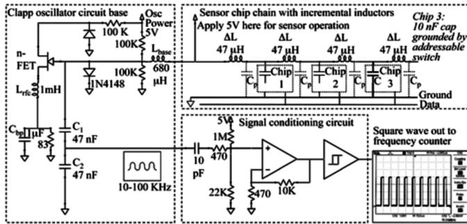
Fig. 1. Oscillator, sensors, and signal conditioning circuit.
