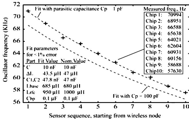
Fig. 2. Oscillator frequency versus sensor position along chain.
