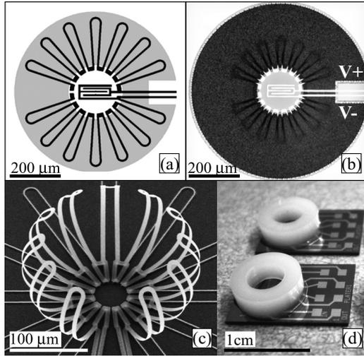
FIG. 2. Released cage devices used for bubble generation and trapping.
