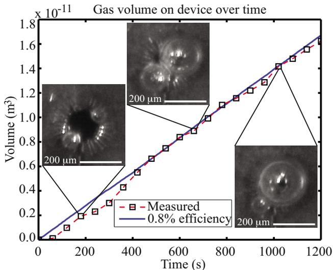
FIG. 3. (Color online) Measured bubble volume present over 20 min plotted beside the ideal gas generation at 0.8%
