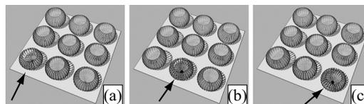
FIG. 1. Array of 300  $\mu\text{m}$  diameter bubble traps undergoing an electroplating sample collection sequence across the front row.
