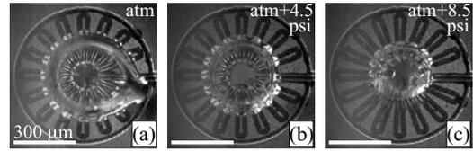
FIG. 4. An air bubble trapped in a microcage in water. The filaments conform to the surface of the bubble over a range of bubble diameters. The outline of the original etch pattern remains on the plane of the substrate, while filaments fold around the bubble.
