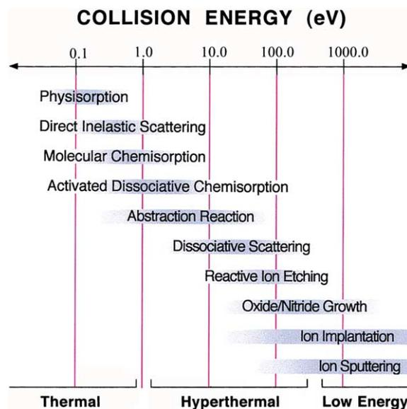
Fig. 1. Fundamental molecule/surface processes: Each shaded region designates the ion kinetic energy range over which the associated process is studied. Adapted from Ref. [150].
