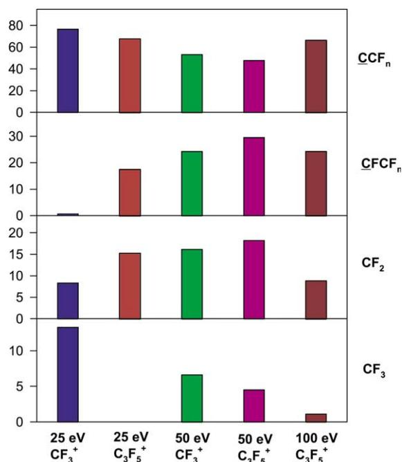
Fig. 5. Chemical composition of polystyrene thin films modified by 25–100 eV  $\text{CF}_3^+$  and  $\text{C}_3\text{F}_5^+$  ion beams, prepared with ion doses equivalent to  $1.5 \times 10^{16}$  F atoms/cm<sup>2</sup>. The percentages of each fluorocarbon component are normalized by removal of the non-fluorocarbon component. These fluorocarbon films are several nm thick and 30–60% fluorine, with the remaining composition carbon. Figure adapted from Ref. [75].
