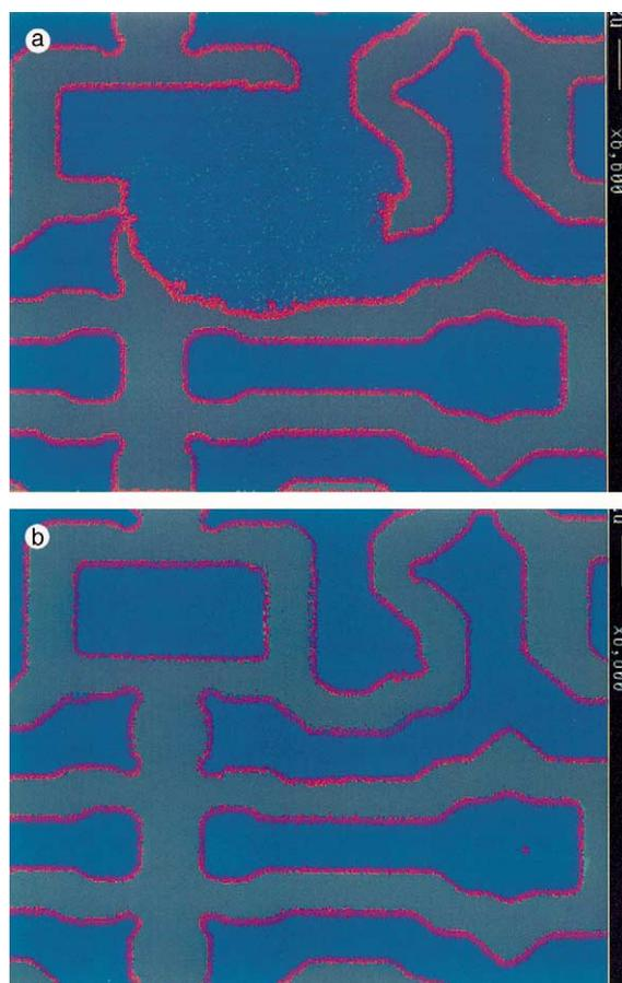
Fig. 8. Panel (a) shows a photomask with Cr features displayed as blue and glass features as either gray or pink when adjacent to Cr (bar at right =  $2 \mu\text{m}$  length). A large blue feature corresponding to extraneous Cr dominates the upper center. Panel (b) shows the same photomask following repair with the  $Ga^+$  ion beam: the extraneous Cr feature is now missing and has been replaced with the correct Cr/glass pattern.
