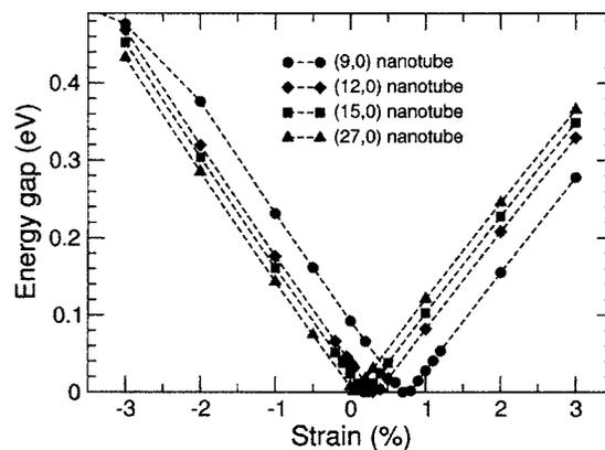
FIG. 2. Calculated energy-gap variation of zigzag (9,0), (12,0), (15,0), and (27,0) SWNTs as a function of axial strain.
