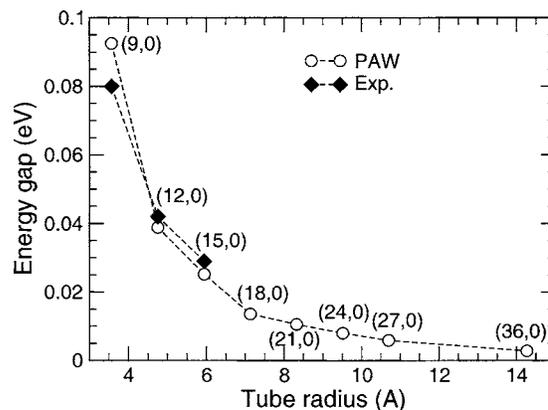
FIG. 1. Calculated (open circles) and experimental (solid diamonds) (Ref. 12) energy gaps of unstrained zigzag semimetallic SWNTs vs their radii.
