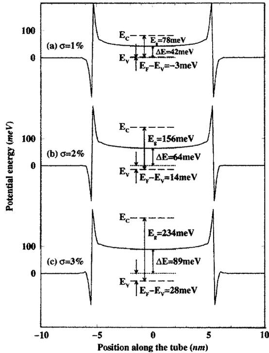
FIG. 3. Self-consistently determined potential energy of zigzag (12,0) SWNT as a function of the atomic position along the tube for (a) strain  $\sigma = 1\%$ , (b)  $\sigma = 2\%$ , and (c)  $\sigma = 3\%$ , respectively. The calculated Fermi levels for the three cases are shown being pinned near the top of the valence band.
