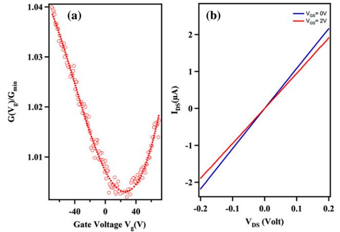
**Figure 4.** (a) The conductance normalized to the minimum conductance,  $G(V_g)/G_{\min}$  versus  $V_g$  of the monolayer graphene FET under ambient conditions. We found our graphene FET to be p-type with net charge  $n_0 > 0$ . (b) Drain–source current ( $I_{DS}$ ) versus the drain–source voltage ( $V_{DS}$ ) under different gate voltages ( $V_g = 0, 2$  V).
