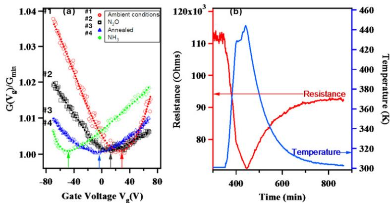
**Figure 5.** (a) Gate voltage dependence of conductivity caused by graphene under ambient conditions (red #1), after vacuum annealing at  $\sim 180^\circ\text{C}$  at  $\sim 2 \times 10^{-7}$  Torr (blue #3), upon exposure to 1 atm ammonia (green #4) and nitrous oxide (black #2).  $V_{\text{DS}} = 200$  mV. (b) The time evaluation of the source–drain resistance and corresponding temperature during the vacuum annealing process at  $V_g = 0$  V.
