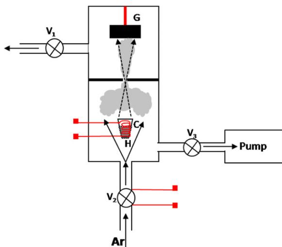
**Figure 1.** The schematics of the gas jet impactor. Metal clusters reaching graphite through the orifice impact the graphite surface and produce different forms of surface distortions including dislocation lines and nano-craters.
