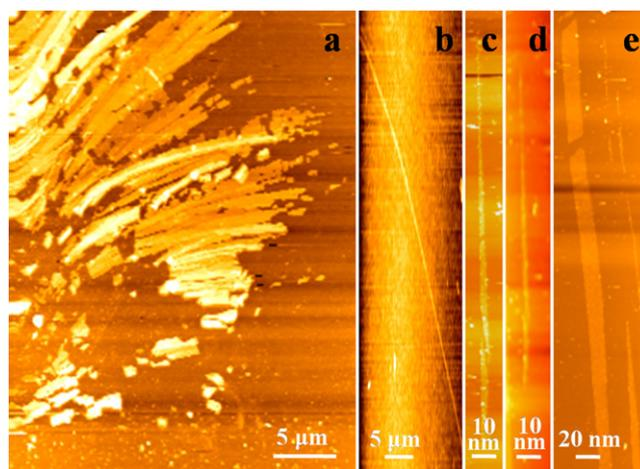
**Figure 2.** AFM images of the graphene ribbons produced by cluster collision. (a) A dense region of dislocation ribbons directed radially around the center of the collision region. (b)–(e) Long individual graphene nano-ribbons (GNRs) transferred to the Si/SiO<sub>2</sub> substrate.
